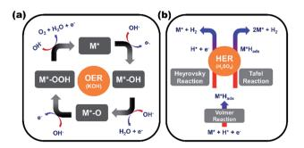
Fig. 5 Probable electrocatalytic mechanism for (a) oxygen evolution reaction (OER) and (b) hydrogen evolution reaction (HER) ( $M^* =$  active site of electrocatalyst;  $H_{abs} =$  adsorbed hydrogen).
