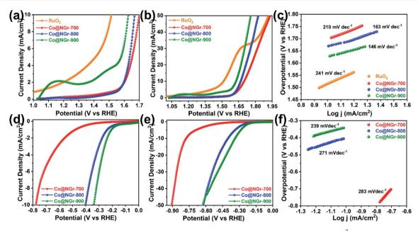
Fig. 4 (a-c) LSV plots and Tafel plots (OER) of Co@NGr-700/800/900 nanomaterials and RuO₂ at 10/50 mA cm²; (d-f) LSV plots and Tafel plots (HER) of Co@NGr-700/800/900 nanomaterials at -10/-50 mA cm<sup>-2</sup>.
