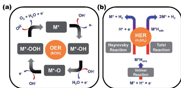
Fig. 5 Probable electrocatalytic mechanism for (a) oxygen evolution reaction (OER) and (b) hydrogen evolution reaction (HER) ( $\text{M}^*$  = active site of electrocatalyst;  $\text{H}_{\text{ads}}$  = adsorbed hydrogen).
