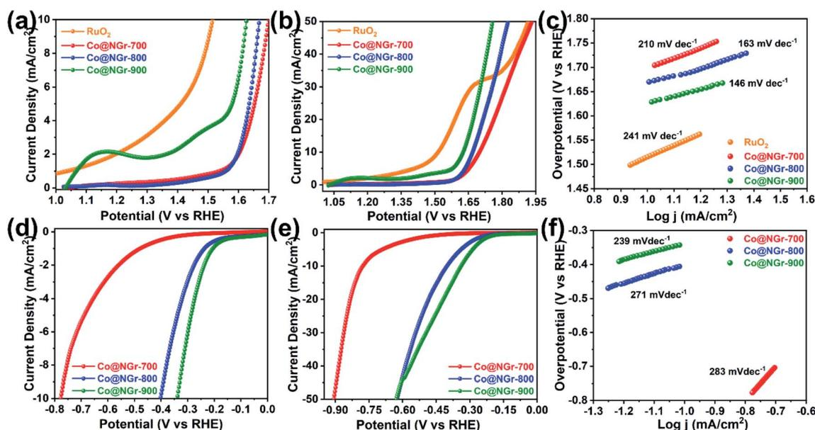
Fig. 4 (a–c) LSV plots and Tafel plots (OER) of Co@NGr-700/800/900 nanomaterials and  $\text{RuO}_2$  at  $10/50 \text{ mA cm}^{-2}$ ; (d–f) LSV plots and Tafel plots (HER) of Co@NGr-700/800/900 nanomaterials at  $-10/-50 \text{ mA cm}^{-2}$ .
