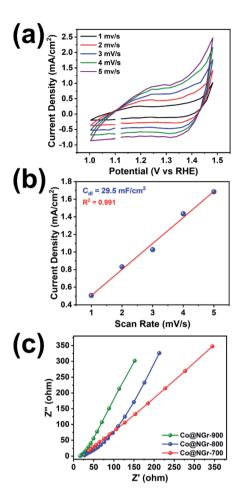
**Fig. 6** (a) CV for Co@NGr-900 at different scan rates vs. RHE; (b) the linear fitting of current density at 1.43 V vs. RHE vs. different scan rates for Co@NGr-900; (c) Nyquist Plot for Co@NGr-700/800/900 nanomaterials.
