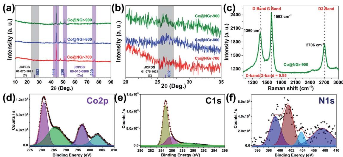
Fig. 3 (a and b) PXRD patterns of Co@NGr-700/800/900 nanomaterials compared with graphitic carbon and metallic cobalt JCPDS reference patterns; (c) FT-Raman spectrum of Co@NGr-900; (d–f) High resolution XPS spectrum of Co@NGr-900 for Co 2p, C 1s and N 1s.
