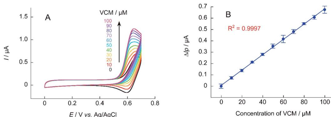
Fig. 10 (A) Cyclic voltammograms of A-TEMPO (0.1 mM) in the absence and presence of VCM (10–100  $\mu\text{M}$ ) in 100 mM phosphate buffer (pH 7.4); scan rate: 10  $\text{mV s}^{-1}$ . (B) Calibration curve of  $\Delta I_p$  for VCM concentration obtained from cyclic voltammetry.
