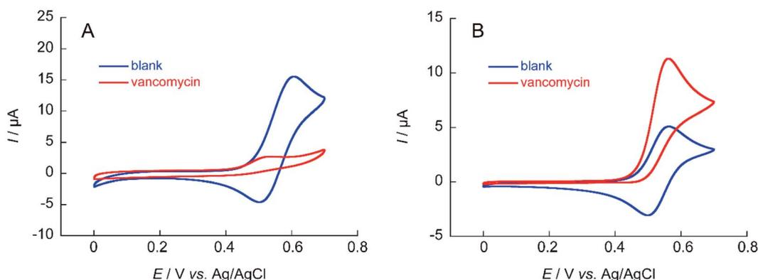
Fig. 8 Cyclic voltammograms of (A) 1 mM NNO and (B) 1 mM TEMPO in the absence and presence of 1 mM VCM in 100 mM phosphate buffer (pH 7.4); scan rate: (A) 100  $\text{mV s}^{-1}$ , (B) 10  $\text{mV s}^{-1}$ .
