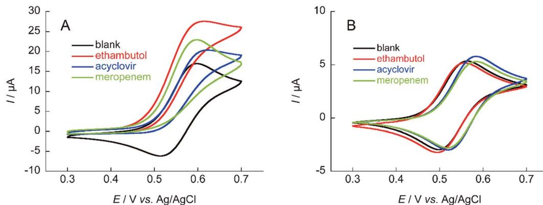
Fig. 4 Cyclic voltammograms of (A) 1 mM NNO and (B) 1 mM TEMPO in the absence and presence of 1 mM ethambutol, acyclovir, and meropenem in 100 mM phosphate buffer (pH 7.4); scan rate: (A) 100 mV s<sup>-1</sup>, (B) 10 mV s<sup>-1</sup>.
