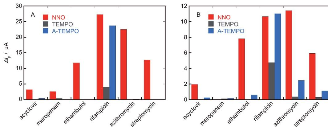
Fig. 11  $\Delta I_p$  values of NNO, TEMPO, and A-TEMPO obtained using each antibiotic as a substrate; scan rate: (A) 100 mV s<sup>-1</sup>, (B) 10 mV s<sup>-1</sup>.
