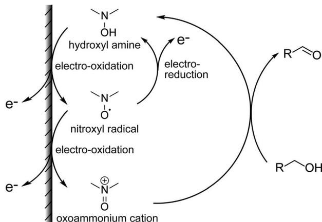
Fig. 1 Electrochemical detection of alcohols using nitroxyl radicals.
