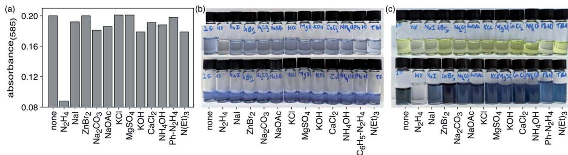
Fig. 5 (a) Absorptivities of DMSO solutions of **1c** ( $4.8 \times 10^{-5}$  M) after addition of various analytes. (b) Changes in the colour of DMSO solutions of **1c** before (top) and after (bottom) addition of various analytes. (c) Changes in the colour of DMSO solutions of before (top) and after (bottom) addition of various analytes and exposure to 312 nm light for 60 s.
