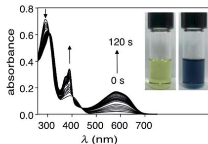
**Fig. 1** Changes in the UV-vis absorption spectra when a  $\text{CHCl}_3$  solution ( $1.0 \times 10^{-5}$  M) of ring-open isomer **1o** is exposed to 312 nm light for 2 minutes. The inset shows the colour change as a result of the photocyclization.
