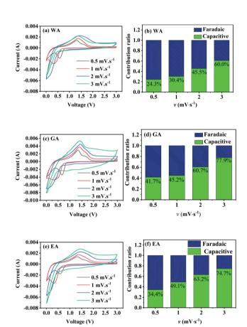
Fig. 10 CV curves and capacitive contributions to the total capacity of the prepared  $MnC_2O_4$  at different sweep rates (v mV s<sup>-1</sup>).
