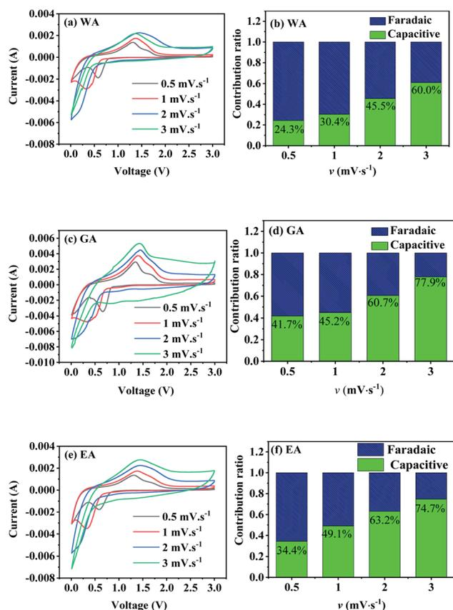
Fig. 10 CV curves and capacitive contributions to the total capacity of the prepared MnC<sub>2</sub>O<sub>4</sub> at different sweep rates ( $v$  mV s<sup>-1</sup>).
