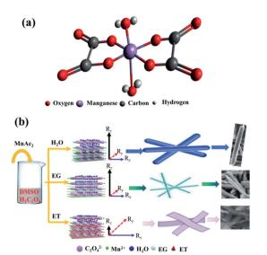
Fig. 8 Schematic illustration of (a) the structure and (b) the formation process of manganese oxalates.  $R_z$  is growth direction vectors perpendicular to the crystal plane, and  $R_x$  and  $R_y$  are growth direction vectors parallel to the crystal plane.
