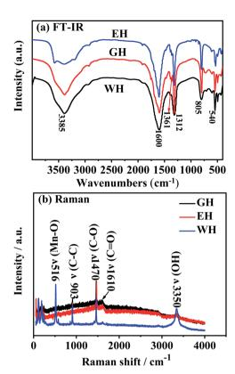
Fig. 3 (a) FT-IR spectra and (b) Raman spectra for the precursors prepared in  $H_2O$ -DMSO, ET-DMSO and EG-DMSO.
