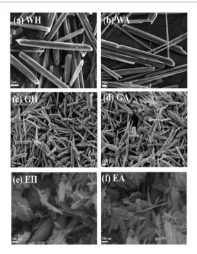
**Fig. 5** SEM images of the prepared precursors in different solvents (a, c and e) and the corresponding dehydration products (b, d and f).
