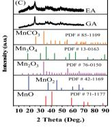
Fig. 1 XRD patterns: (a) precursors, (b) dehydrated products prepared in different solvents, and (c) comparison with other Mn-based
