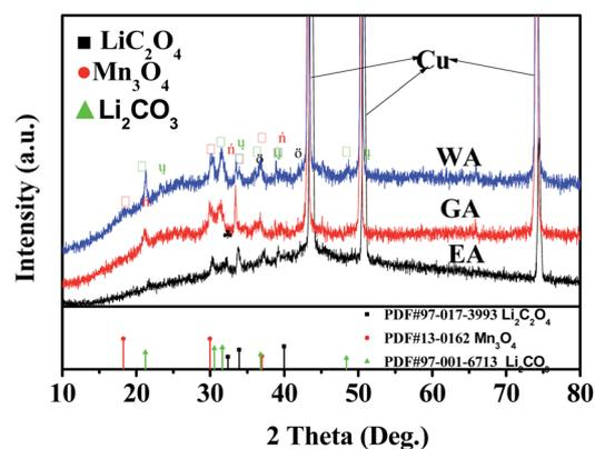
Fig. 12 XRD for the prepared samples after 600 cycles at 20C.
