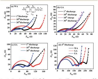
Fig. 13 Nyquist plots of MnC<sub>2</sub>O<sub>4</sub> prepared by different solvents at 3C: (a) WA, (b) GA, (c) EA, and (d) 4th discharge.
