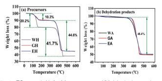
Fig. 4  $\,$  TG curves in  $\,$  N $_{2}$  for (a) precursors, and (b) dehydration products.
