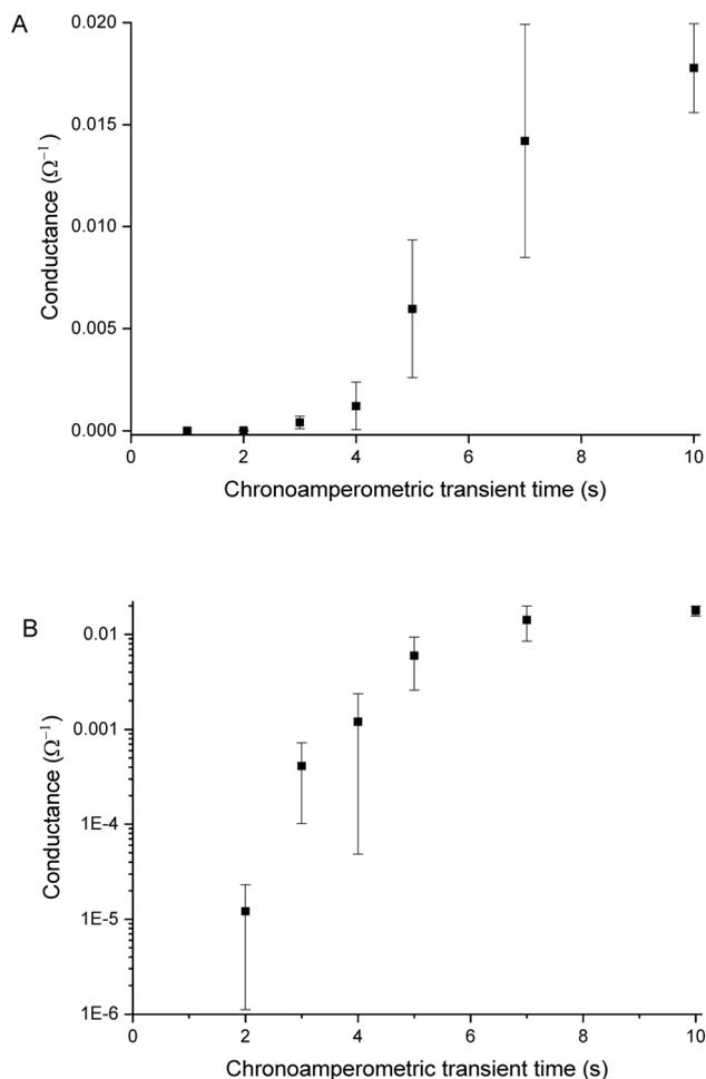
**Fig. 4** Conductance vs. chronoamperometric deposition time for PEDOT on glass substrates with Pt interdigitated electrodes with a 5  $\mu\text{m}$  separation (A). The conductance increases with increasing deposition time. Plotting the same data in a semi-logarithmic plot highlights the large change in conductance caused by depositing slightly more polymer in the percolation region between 2 and 7 s (B). The error bars represent the standard deviation of 3 independent experiments.
