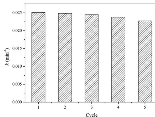
Fig. 11 Recycling test of TS-2 in VUV/TS-2 process. [UDMH]<sub>0</sub> = 100 mg L<sup>-1</sup>, pH<sub>0</sub> = 9.0, *T* = 30 °C.
