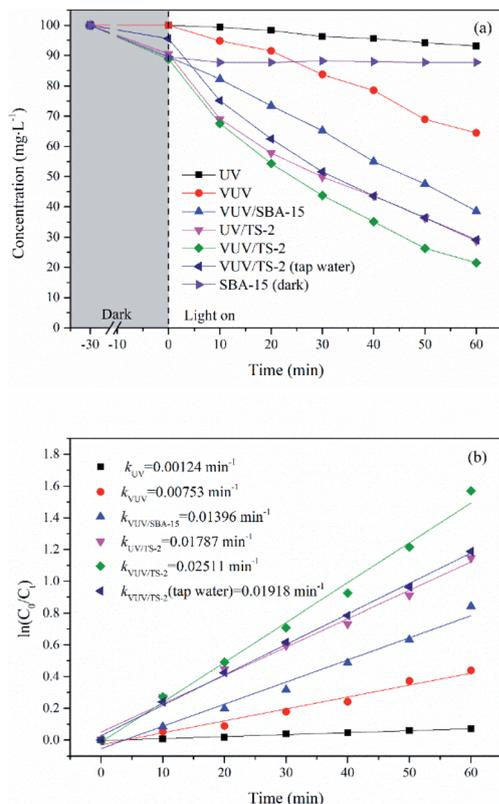
Fig. 8 Time course of UDMH concentration in different process (a) and rate constant of UDMH degradation (b). [UDMH]<sub>0</sub> = 100 mg L<sup>-1</sup>, pH<sub>0</sub> = 9.0, T = 30 °C.
