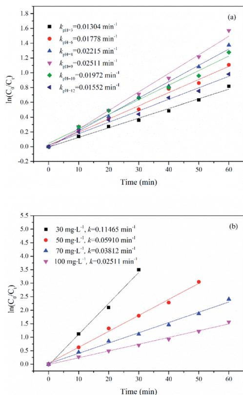
Fig. 10 Effect of initial pH (a) and initial substrate concentration (b) on the degradation of UDMH in VUV/TS-2 process. (a) [UDMH]<sub>0</sub> = 100 mg L<sup>-1</sup>, *T* = 30 °C; (b) pH<sub>0</sub> = 9.0, *T* = 30 °C.
