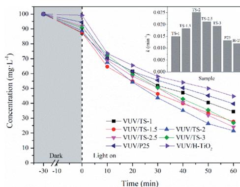
Fig. 9 Time course of UDMH concentration over TiO<sub>2</sub>/SBA-15 with different Ti contents in VUV process, with the rate constants (inset). [UDMH]<sub>0</sub> = 100 mg L<sup>-1</sup>, pH<sub>0</sub> = 9.0, T = 30 °C.
