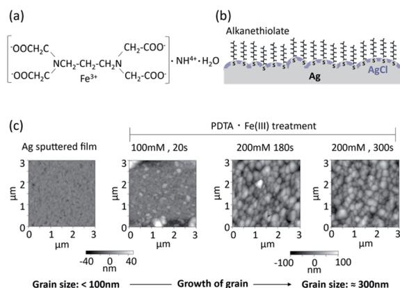
Fig. 1 Surface morphology of silver chloride layer prepared by chemical deposition using PDTA·Fe(III). (a) Chemical formula of PDTA·Fe(III); (b) conceptual structure of the organic and inorganic mixed phase modification of a silver surface; (c) AFM images of silver chloride surfaces prepared with PDTA·Fe(III) on a sputtered silver thin film.
