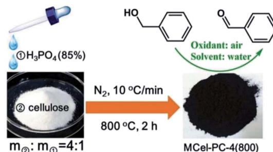
Fig. 32 Preparation of M Cel-PC4(800) and catalytic application in oxidation of benzyl alcohol. Reprinted with permission from ref. 241. Copyright 2018 Royal Society of Chemistry.
