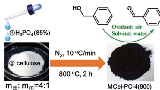
Fig. 32 Preparation of M Cel-PC4(800) and catalytic application in oxidation of benzyl alcohol. Reprinted with permission from ref. 241. Copyright 2018 Royal Society of Chemistry.
