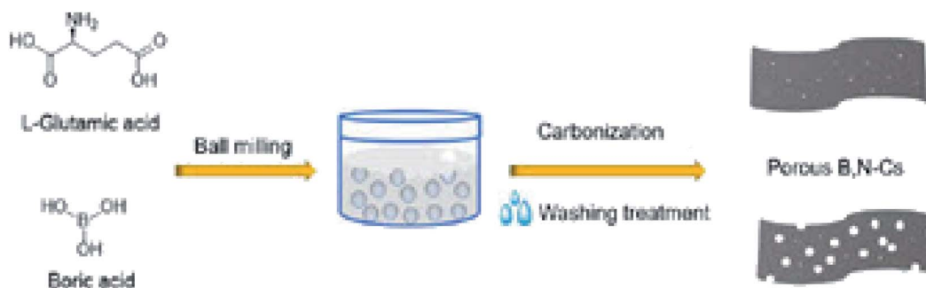
Fig. 47 Preparation of porous B,N-Cs. Reprinted with permission from ref. 260. Copyright 2020 John Wiley and Sons.
