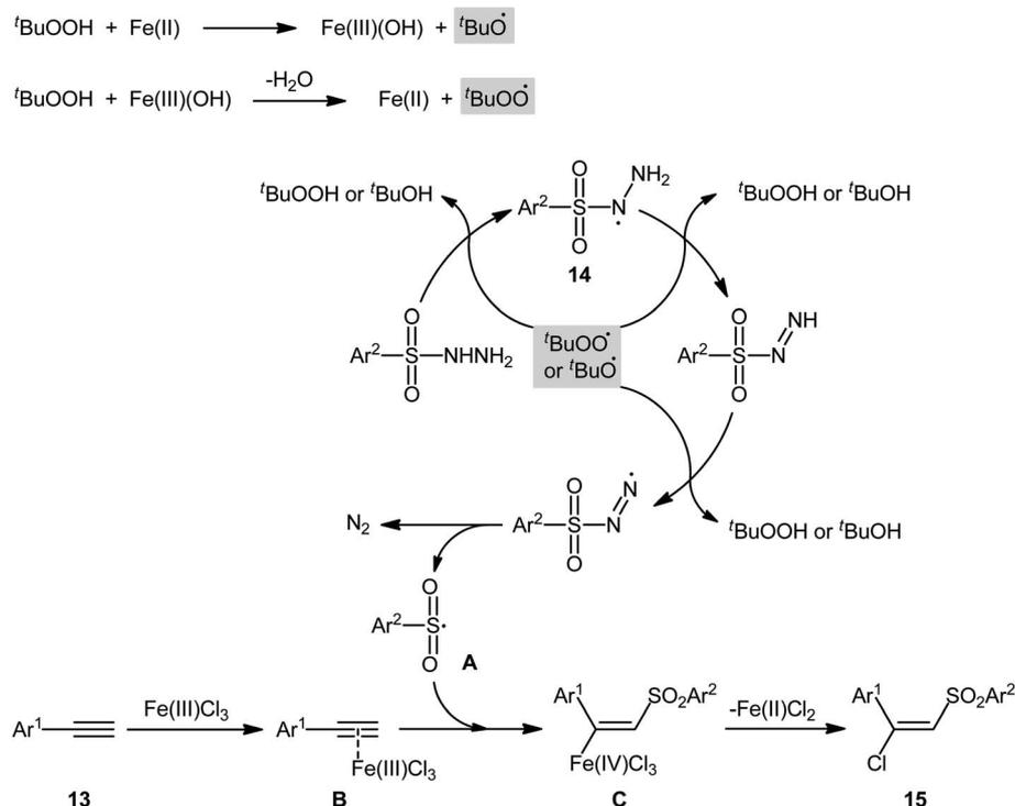
Scheme 7 Proposed Mechanism for the reaction in Scheme 6.
