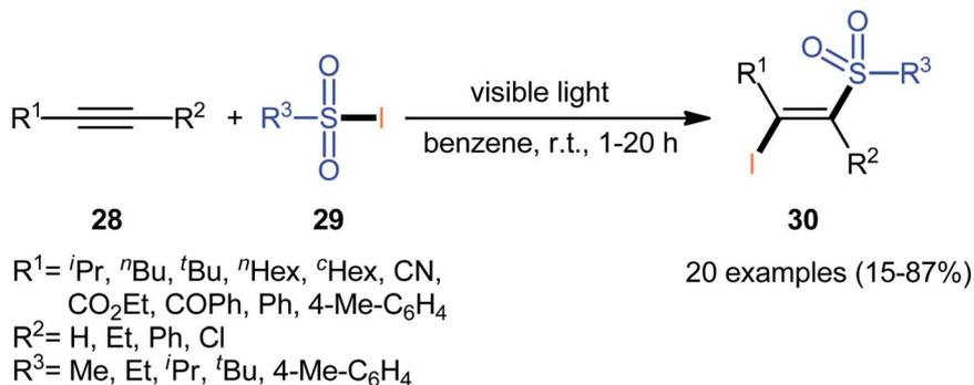
Scheme 13 Truce's synthesis of (*E*)- $\beta$ -iodovinyl sulfones 30.
