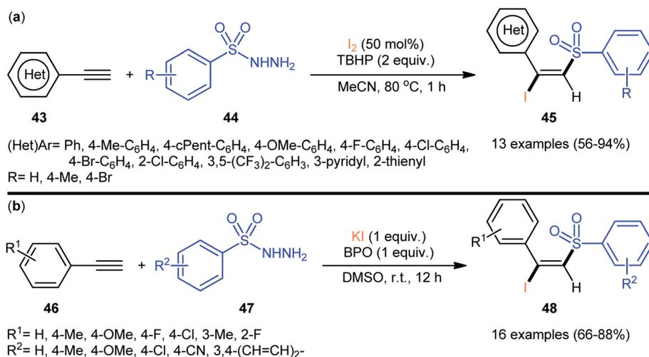
Scheme 20 (a) TBHP-mediated iododisulfonation of terminal alkynes **43** with arylsulfonyl hydrazides **44** and I<sub>2</sub>; (b) BPO-mediated three-component reaction between alkynes **46**, arylsulfonyl hydrazides **47**, and KI.
