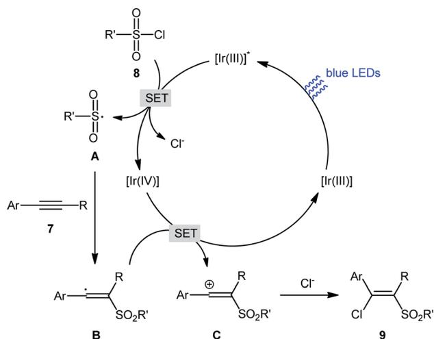
Scheme 4 Mechanistic explanation for the reaction in Scheme 3.
