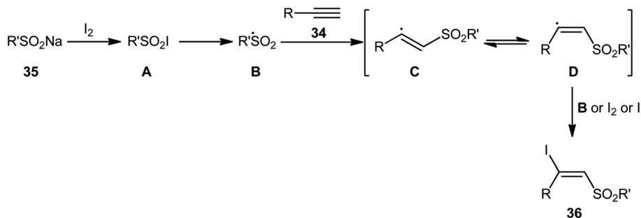
Scheme 16 A proposed pathway for the formation of (*E*)-β-iodovinyl sulfones **36**.
