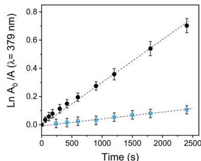
Fig. 5 First-order kinetic data fitting for the photooxidation of DMA in DMF sensitized by PEDOT-C<sub>60</sub> (■) and fullerene C<sub>60</sub> (●).  $\lambda_{\text{irr}} = 455\text{--}800 \text{ nm}$ . Values represent mean  $\pm$  standard deviation (error bars) of three consecutive experiments.
