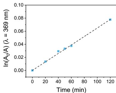
Fig. 4 First-order plot for the photodegradation of PEDOT-C<sub>60</sub> surface dipped in PBS and irradiated with visible light.
