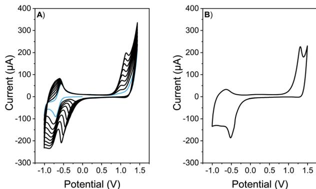
Fig. 1 (A) Repetitive cyclic voltammograms of a 0.5 mM solution of EDOT-C<sub>60</sub> in TBAPF<sub>6</sub> (0.1 M)/DCM. Light blue line denotes the first cyclic voltammogram. (B) Cyclic voltammogram of a PEDOT-C<sub>60</sub> film electro-deposited on ITO electrode in TBAPF<sub>6</sub> (0.1 M)/DCM. Scan rate: 50 mV s<sup>-1</sup>.
