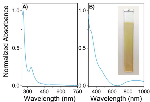
Fig. 3 (A) Electronic absorption spectrum of **EDOT-C<sub>60</sub>** monomer in DCM at room temperature. (B) Absorption spectrum of **PEDOT-C<sub>60</sub>** film on ITO. The inset shows a photo of the polymer **PEDOT-C<sub>60</sub>** deposited on ITO.
