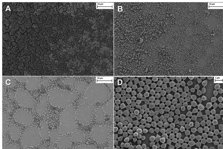
Fig. 11 SEM images of *S. aureus* biofilm on PEDOT-C<sub>60</sub>. (A) Control: *S. aureus* biofilm on PEDOT-C<sub>60</sub> keeping in the dark; (B) *S. aureus* biofilm on PEDOT-C<sub>60</sub> exposed to visible light for 30 min; (C) *S. aureus* biofilm on PEDOT-C<sub>60</sub> exposed to visible light for 60 min; (D) *S. aureus* biofilm on PEDOT-C<sub>60</sub> exposed to visible light for 60 min at a higher magnification.
