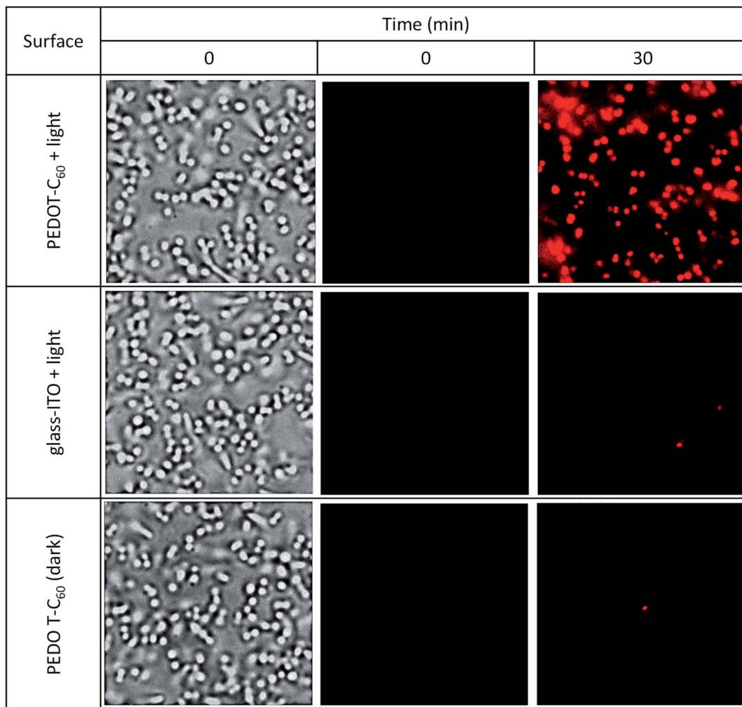
Fig. 9 Bright-field (first column) and fluorescence microscopy (second and third columns) images of *S. aureus* on the surface of a coverslip coated with PEDOT-C<sub>60</sub> + light and the controls, ITO with no coating + light and a PEDOT-C<sub>60</sub> surface in the dark. [PI] = 1 μM. Light dose: 5.6 J cm<sup>-2</sup>.
