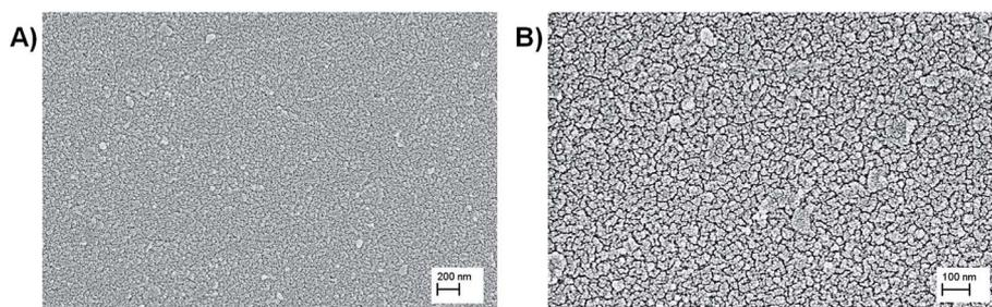
Fig. 2 SEM images of PEDOT-C<sub>60</sub> polymer film at different magnifications: (a) 23 000 $\times$ , and (b) 57 000 $\times$ .
