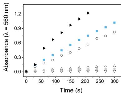
Fig. 6 O<sub>2</sub><sup>•-</sup> generation monitored by the NBT method following the increase in the absorption at 560 nm. Samples contain: PEDOT-C<sub>60</sub>, NBT and NADH (■); fullerene C<sub>60</sub> solution, NBT and NADH (▲); NBT and NADH (○); PEDOT-C<sub>60</sub> and NBT (△); PEDOT-C<sub>60</sub> and NADH (▽); PEDOT-C<sub>60</sub>, NBT and NADH, dark control (◆). [NBT] = 0.2 mM and [NADH] = 0.5 mM.
