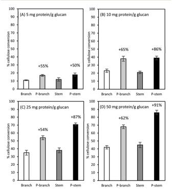
Fig. 3 Percent cellulose conversion to glucose for unpretreated and pretreated hemp materials at a different enzyme dosage of Cellic CTec2 cellulase: (A) 5 mg protein per g glucan, (B) 10 mg protein per g glucan, (C) 25 mg protein per g glucan, and (D) 50 mg protein per g glucan. Cellulose in 1% (w/v) glucan solids was hydrolyzed in a 50 mL agitated flask at 50 °C for 72 h. All tests were run in duplicate and the average is presented. P-stem: pretreated stem; P-branch: pretreated branch.
