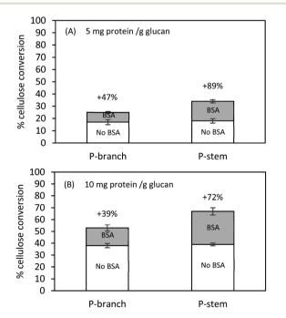
Fig. 4 Cellulose conversion of pretreated and washed hemp solids at 1% (w/v) glucan in the presence of 5 or 10 mg protein per g glucan with or without supplementation. Hydrolysis was conducted in a 50 mL flask agitated (250 rpm) at 50 °C for 72 h. All tests were completed in duplicate with a 95% significant difference.
