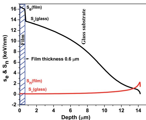
Fig. 1 Variation of the electronic energy loss  $S_e$  and the nuclear energy loss  $S_n$  of 120 MeV Ag ions with depth as the ions traverse the thickness of the AgInSe<sub>2</sub> thin films.
