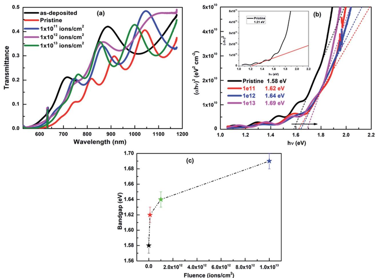
Fig. 5 (a) Transmittance spectra of the as-deposited amorphous film, annealed film, and 120 MeV Ag irradiated film at fluences  $1 \times 10^{11}$ ,  $1 \times 10^{12}$ , and  $1 \times 10^{13}$  ion  $\text{cm}^{-2}$  (b)  $h\nu$  vs.  $(\alpha h\nu)^2$  plot of pristine and irradiated  $\text{AgInSe}_2$  thin films. The inset shows the extraction of the fundamental bandgap of  $\text{AgInSe}_2$  by linear fitting of the oscillatory region. (c) Bandgap variation with fluence.
