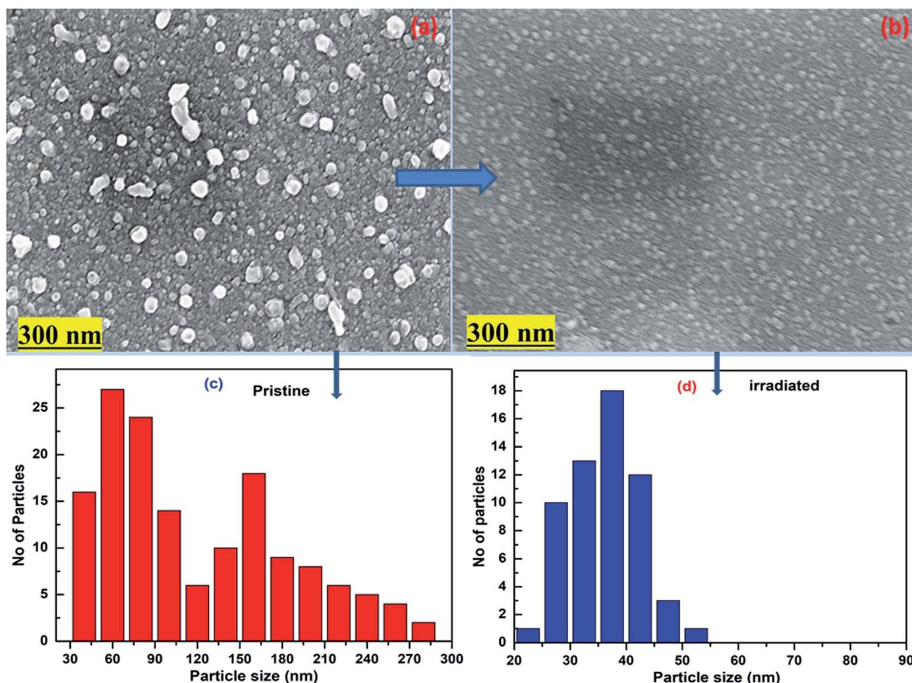
Fig. 4 FESEM images of (a) pristine and (b)  $1 \times 10^{13}$  ions per cm<sup>2</sup> fluence irradiated AgInSe<sub>2</sub> thin films (c) histogram of AgInSe<sub>2</sub> pristine thin films and (d) histogram of 120 MeV Ag ion irradiated film at the fluence of  $1 \times 10^{13}$  ions per cm<sup>2</sup>.
