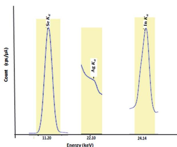
Fig. 2 The line scans of Se  $K_{\alpha}$ , Ag  $K_{\alpha}$ , and In  $K_{\alpha}$  in the EDXRF spectrum of pristine AgInSe<sub>2</sub> thin film.
