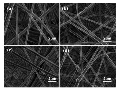
Fig. 8 SEM of fibrous membrane after formaldehyde filtration ((a) is 0 wt%, (b) is 1 wt%, (c) is 3 wt% and (d) is 5 wt%).
