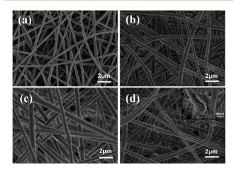
Fig. 2 SEM image of nanofiber membranes ((a) is pure PAN nanofiber membranes; (b) is PAN@g- $C_3N_4$  nanofiber membrane with 1 wt% g- $C_3N_4$ ; (c) is PAN@g- $C_3N_4$  nanofiber membrane with 3 wt% g- $C_3N_4$ ; (d) is PAN@g- $C_3N_4$  nanofiber membrane with 5 wt% g- $C_3N_4$  and the local amplified view).
