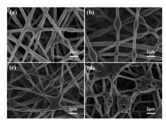
Fig. 5 SEM of nanofibrous membrane with a  $g-C_3N_4$  addition of 3 wt% filtering polluted air at different duration ((a) is 1 h, (b) is 3 h, (c) is 5 h, (d) is 8 h).
