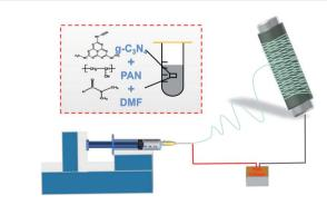
Scheme 1 Mechanism of diagram electrospinning.
