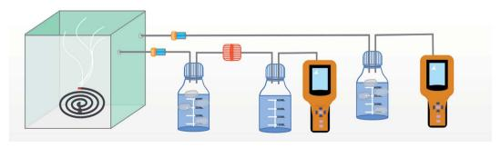
Scheme 2 Mechanism diagram of PM generation and evaluation of the filtering efficiency
