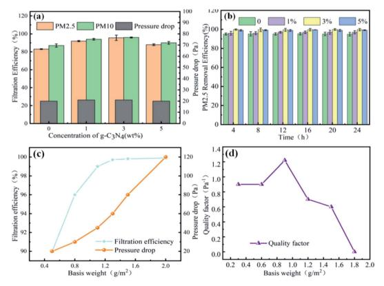
Fig. 4 Filtration performance of the nanofiber membrane ((a) is filtration efficiency and pressure drop with different  $g-C_3N_4$  addition, (b) is filtration stability of PM2.5, (c) is filtration efficiency and pressure drop with different weight, (d) is quality factor).
