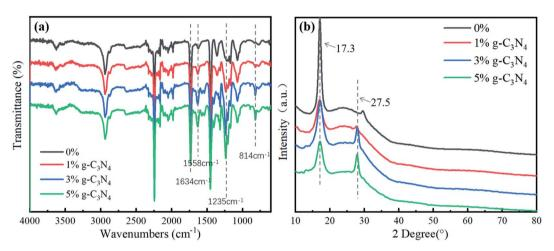
Fig. 1 The FTIR and XRD of nanofibrous membrane ((a) is FTIR and (b) is XRD).
