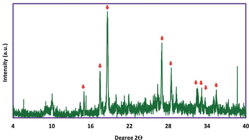
Fig. 1 The PXRD pattern of the synthesized Ni/Zn-BTC bi-MMOF.
