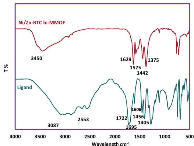
Fig. 2 The FT-IR spectra of the ligand ( $\text{H}_3\text{BTC}$ ) and synthesized Ni/Zn-BTC bi-MMOF.
