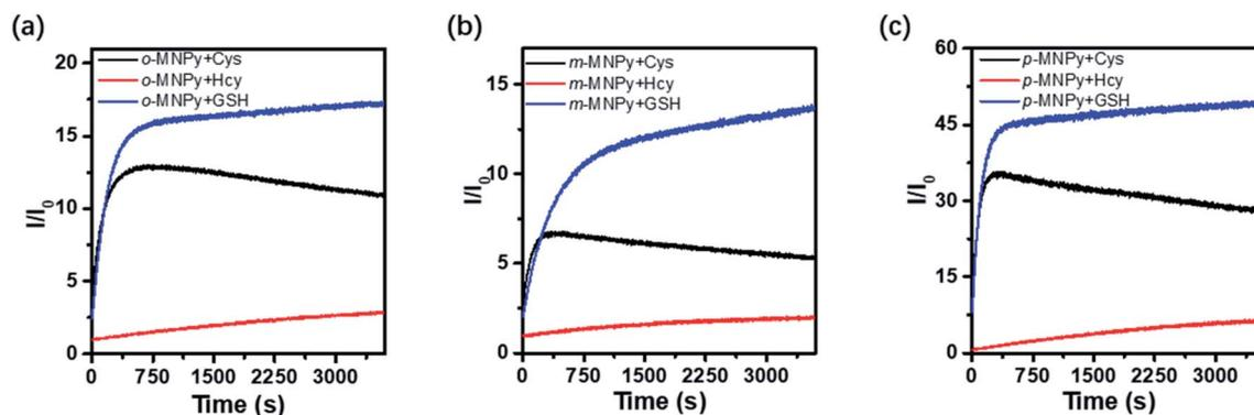
Fig. 2 The time-dependent fluorescence intensity changes of (a) *o*-MNPy, (b) *m*-MNPy and (c) *p*-MNPy in the presence of three biothiols. Concentrations: probe 10 μM, Cys 100 μM, Hcy 10 μM, and GSH 5 mM.
