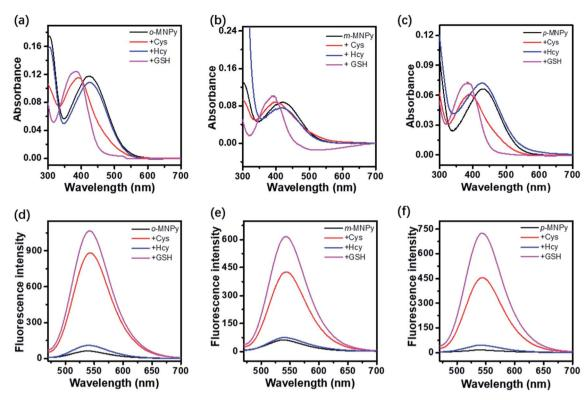
Fig. 1 The UV-vis spectra of (a) o-MNPy, (b) m-MNPy and (c) p-MNPy, and the fluorescence spectra of (d) o-MNPy, (e) m-MNPy and (f) p-MNPy before and after the addition of Cys (100  $\mu$ M), Hcy (10  $\mu$ M) and GSH (5 mM). The concentration of each probe was 10  $\mu$ M in PBS (containing 10% DMSO).
