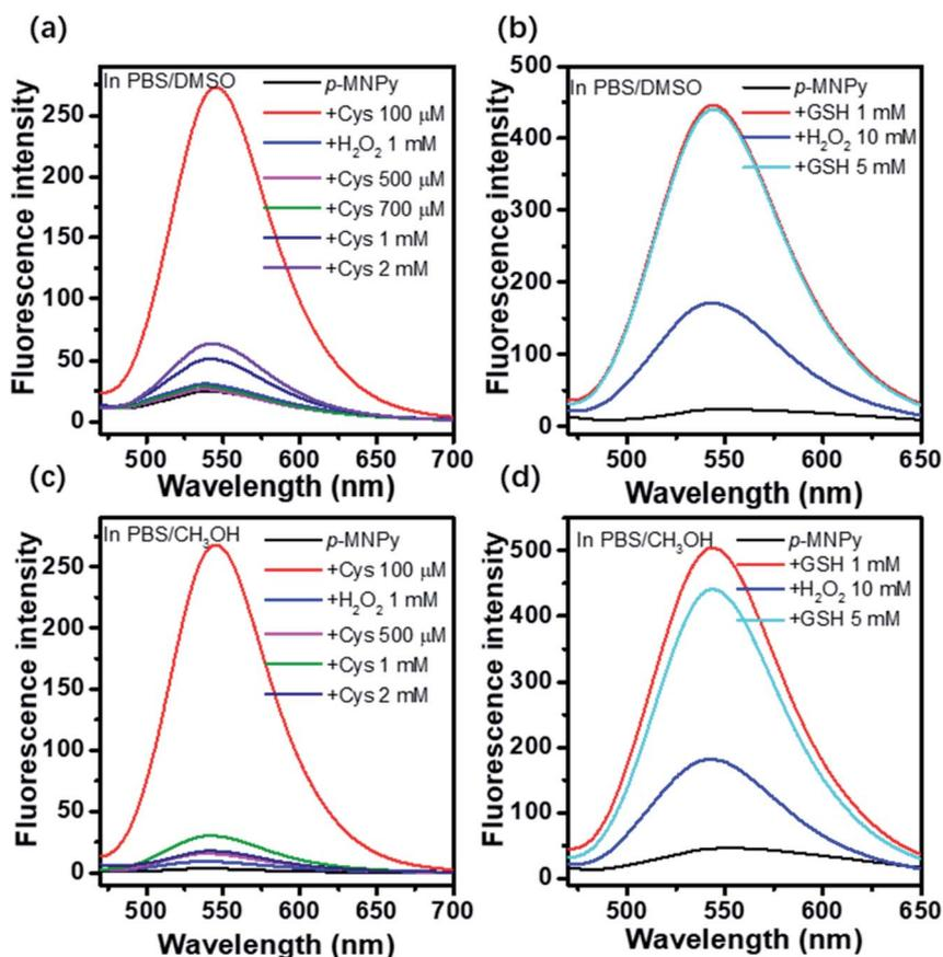
Fig. 5 The fluorescence changes of  $p$ -MNPy with the addition of (a) Cys or (b) GSH and  $\text{H}_2\text{O}_2$  in PBS/DMSO (v/v, 9/1), and with the addition of (c) Cys or (d) GSH and  $\text{H}_2\text{O}_2$  in PBS/ $\text{CH}_3\text{OH}$  (v/v, 8/2).
