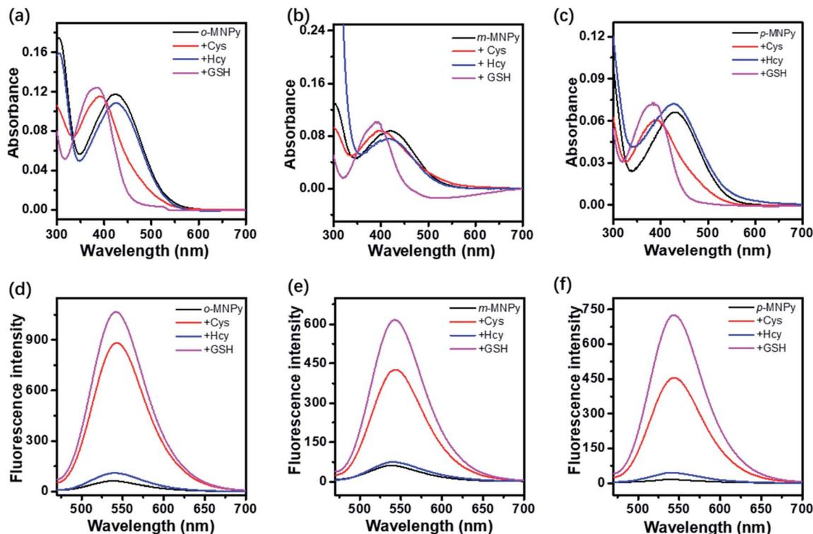
Fig. 1 The UV-vis spectra of (a) *o*-MNPy, (b) *m*-MNPy and (c) *p*-MNPy, and the fluorescence spectra of (d) *o*-MNPy, (e) *m*-MNPy and (f) *p*-MNPy before and after the addition of Cys (100 μM), Hcy (10 μM) and GSH (5 mM). The concentration of each probe was 10 μM in PBS (containing 10% DMSO).
