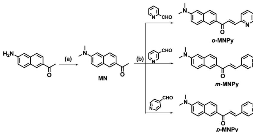
Scheme 2 The synthetic routes of ***o*-MNPY**, ***m*-MNPY** and ***p*-MNPY**. Conditions: (a)  $\text{CH}_3\text{I}$ ,  $\text{K}_2\text{CO}_3$ , DMF, 60 °C; (b) piperidine, acetic acid, ethanol/THF, 80 °C, 96 h.
