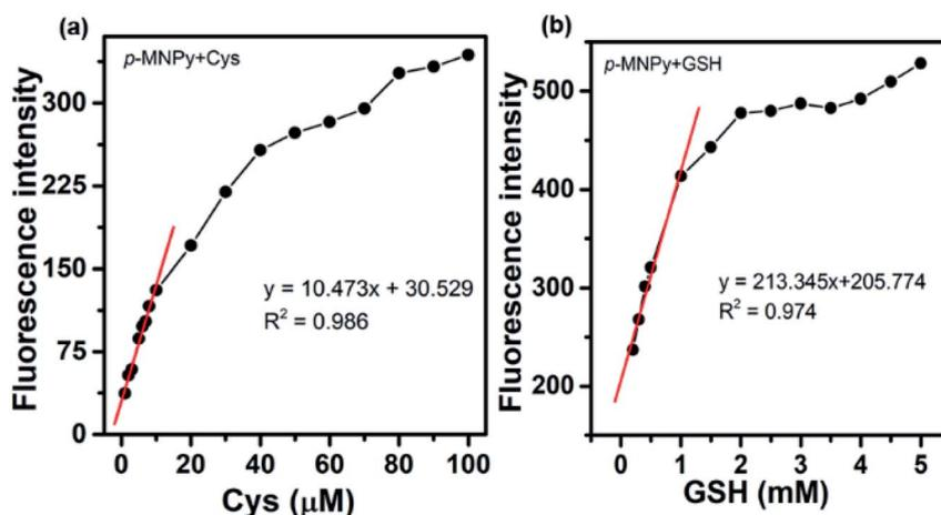
Fig. 3 The changes of fluorescence intensity of *p*-MNPY as the addition of different amount of (a) Cys, and (b) GSH. Concentrations: *p*-MNPY 10  $\mu\text{M}$ , Cys 1–100  $\mu\text{M}$ , GSH 0.1–5 mM.
