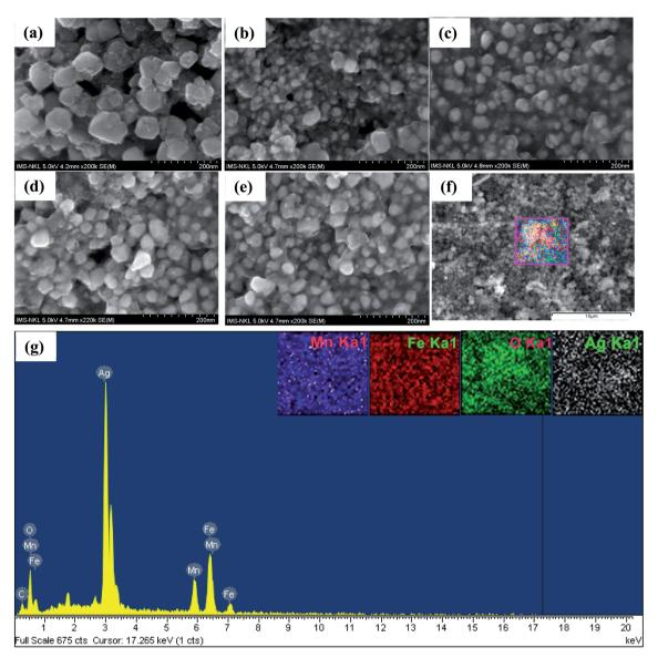
Fig. 3 The SEM micrographs of the heteromeric MnFe<sub>2</sub>O<sub>4</sub>-Ag NPs. (a) S0, (b) S1, (c) and (f) S2, (d) S3, (e) S4. (g) The EDS spectrum of the S2 sample, with the inset showing by color the mappings of the four detected elements for the red dotted box in (f) image.
