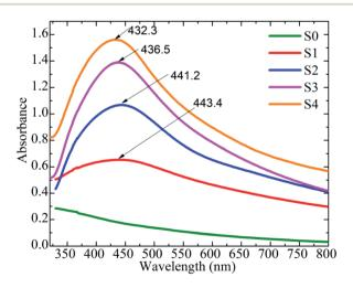
Fig. 6 Room temperature UV-Vis absorbance spectrum of MnFe $_2$ O $_4$ -Ag hybrid NPs.
