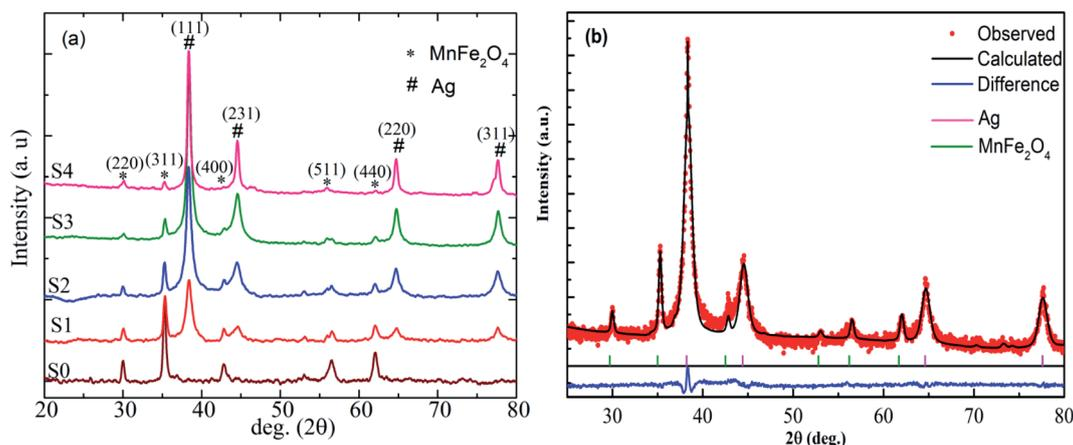
Fig. 2 (a) X-ray diffraction patterns of MnFe<sub>2</sub>O<sub>4</sub>-Ag hybrid NPs. (b) Rietveld fitted room temperature X-ray diffraction patterns for S2 sample.
