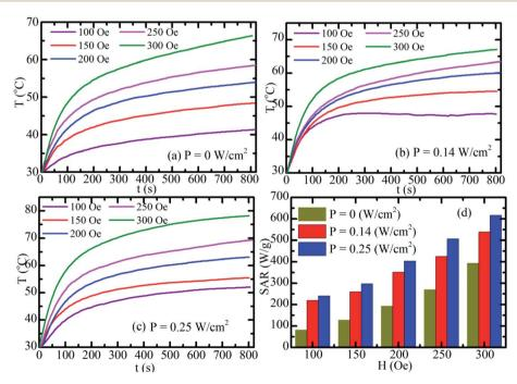
Fig. 10 Time dependent temperature curves of S2 hybrid NPs fluid, gained by synergistic (DUAL) stimulations at various amplitudes of magnetic field under 3 different uses of laser light powers: (a)  $P = 0 \text{ W cm}^{-2}$ , (b)  $P = 0.14 \text{ W cm}^{-2}$ , (c)  $P = 0.25 \text{ W cm}^{-2}$ . (d) The field-dependent SAR values of the S2 hybrid NPs fluid.
