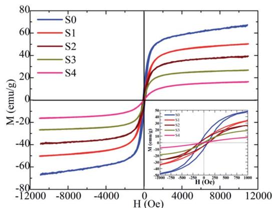
Fig. 8 Room temperature magnetization of  $\text{MnFe}_2\text{O}_4\text{-Ag}$  hybrid NPs.
