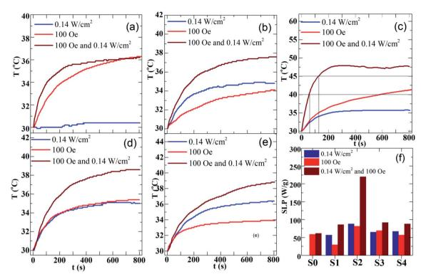
Fig. 9 Photothermal heating and magnetic inductive heating curves of the MnFe<sub>2</sub>O<sub>4</sub>-Ag hybrid nanoparticles suspension (2 mg mL $^{-1}$ ): (a) SO sample, (b) S1 sample, (c) S2 sample, (d) S3 sample and (e) S4 sample. (f) The field-dependent SAR values of the MnFe<sub>2</sub>O<sub>4</sub>-Ag hybrid nanoparticles suspension
