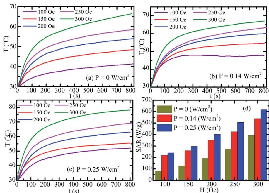
Fig. 10 Time dependent temperature curves of S2 hybrid NPs fluid, gained by synergistic (DUAL) stimulations at various amplitudes of magnetic field under 3 different uses of laser light powers: (a)  $P = 0 \text{ W cm}^{-2}$ , (b)  $P = 0.14 \text{ W cm}^{-2}$ , (c)  $P = 0.25 \text{ W cm}^{-2}$ . (d) The field-dependent SAR values of the S2 hybrid NPs fluid.
