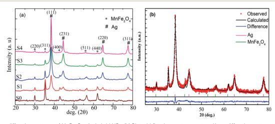
Fig. 2 (a) X-ray diffraction patterns of MnFe $_2$ O $_4$ -Ag hybrid NPs. (b) Rietveld fitted room temperature X-ray diffraction patterns for S2 sample.
