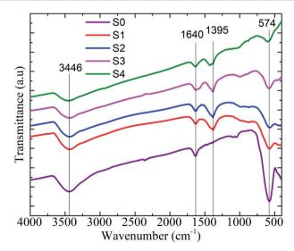
Fig. 5 FT-IR spectra of MnFe<sub>2</sub>O<sub>4</sub>-Ag NPs.
