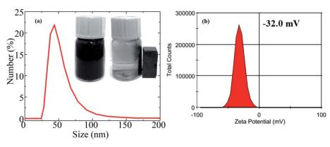
Fig. 11 (a) Dynamic light scattering (DLS) size of MnFe<sub>2</sub>O<sub>4</sub>–Ag hybrid NPs in deionized water. The inset shows the dispersion and separation process of MnFe<sub>2</sub>O<sub>4</sub>–Ag hybrid NPs dispersed from deionized water under an external magnetic field. (b) Z-Potential of MnFe<sub>2</sub>O<sub>4</sub>–Ag hybrid NPs dispersed in water.
