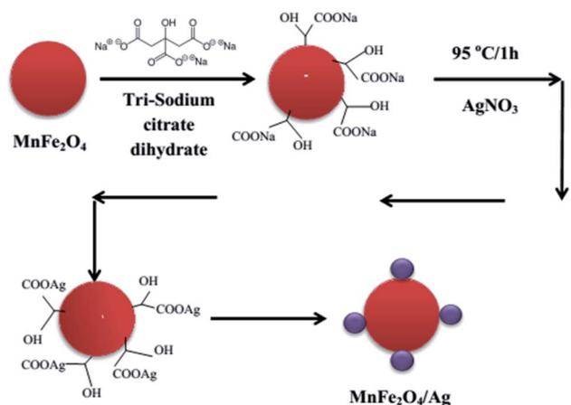
Fig. 1 Schematic diagram of synthesizing  $\text{MnFe}_2\text{O}_4\text{-Ag}$  hybrid NPs.
