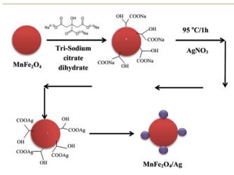
Fig. 1 Schematic diagram of synthesizing MnFe<sub>2</sub>O<sub>4</sub>-Ag hybrid NPs.
