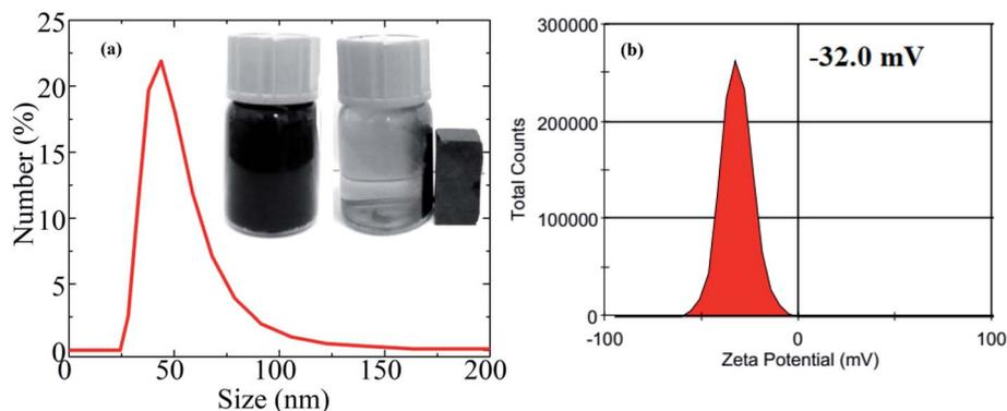
Fig. 11 (a) Dynamic light scattering (DLS) size of  $\text{MnFe}_2\text{O}_4\text{-Ag}$  hybrid NPs in deionized water. The inset shows the dispersion and separation process of  $\text{MnFe}_2\text{O}_4\text{-Ag}$  hybrid NPs dispersed from deionized water under an external magnetic field. (b) Z-Potential of  $\text{MnFe}_2\text{O}_4\text{-Ag}$  hybrid NPs dispersed in water.
