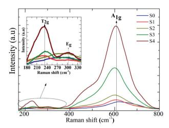
Fig. 7 Room temperature Raman spectra of pure and  $MnFe_2O_4$ -Ag nanoparticles.
