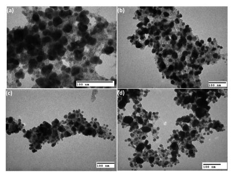
Fig. 4 Typical TEM images of the MnFe<sub>2</sub>O<sub>4</sub>-Ag nanoparticles synthesized with (a) 2:1, (b) 1:1, (c) 1:2 and (d) 1:2.5 mass ratios of MnFe<sub>2</sub>O<sub>4</sub> and Ag.
