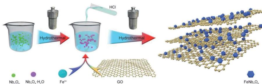
Scheme 1 Schematic illustration of the process for fabricating FNO/rGO composite.
