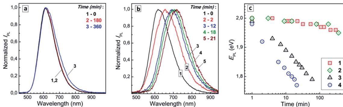
**Fig. 4** Normalized PL spectra of a concentrated 1 : 1 mixture of colloidal AIS and CIS QDs kept at 25 °C (a) and 96–98 °C (b). (c) Evolution of PL band maximum energy ( $E_{\text{PL}}$ ) for diluted (1 and 3) and concentrated (2 and 4) mixtures of colloidal AIS and CIS QDs kept at 25 °C (1 and 2) and 96–98 °C (3 and 4).
