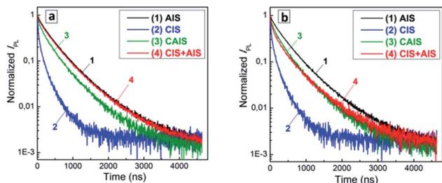
**Fig. 3** Kinetic curves of PL decay registered in the PL band maxima for AIS QDs (curves 1), CIS QDs (2), CAIS QDs (3), and 1 : 1 mixtures of AIS and CIS QDs (4) kept for 60 min at 25 °C (a) and 96–98 °C (b).
