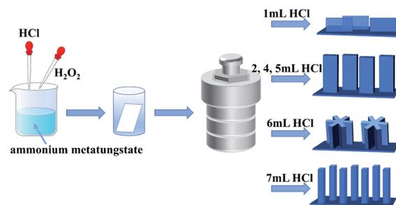
Fig. 3 Schematic of the  $\text{WO}_3$  arrays on FTO.
