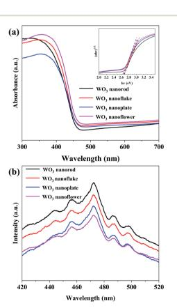
Fig. 5 (a) UV-Vis absorption spectra and (b) room temperature PL spectra of the annealed  $WO_3$  arrays.
