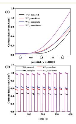
Fig. 6 (a) Linear sweep voltammetry (LSV) curves of the  $WO_3$  arrays. (b) Amperometric I-t curve of the  $WO_3$  arrays at 1.2 V vs. RHE.
