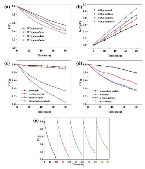
Fig. 7 (a) PC degradation of MB and (b) the corresponding kinetic curves by different  $WO_3$  morphology films. (c) Degradation of MB *via* various techniques using  $WO_3$  nanoflowers. (d) Photocatalytic degradation of MB over  $WO_3$  nanoflowers using different scavengers. (e) Durability of the  $WO_3$  nanoflower photoanode for the degradation of MB.
