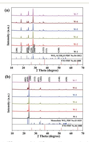
Fig. 4 XRD patterns of the  $WO_3$  arrays (a) as-prepared and (b) annealed.
