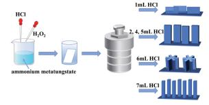
Fig. 3 Schematic of the WO<sub>3</sub> arrays on FTO.
