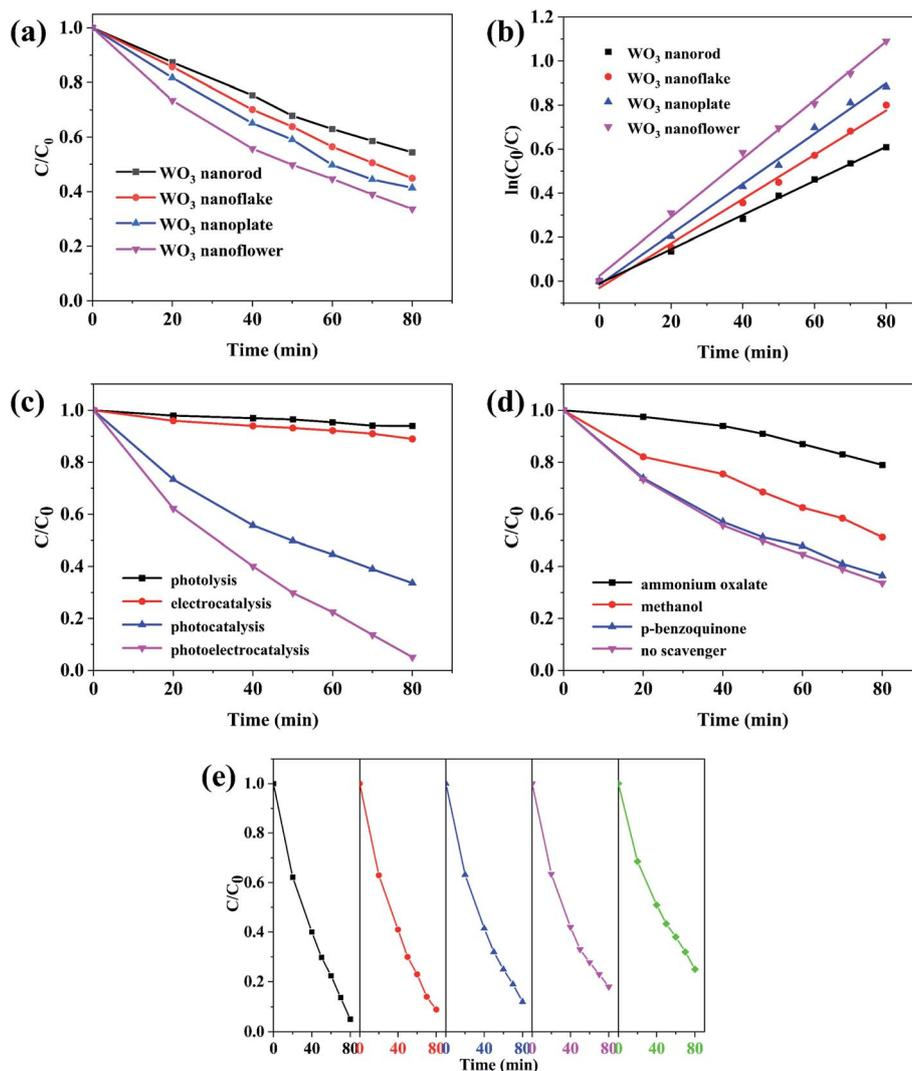
Fig. 7 (a) PC degradation of MB and (b) the corresponding kinetic curves by different  $\text{WO}_3$  morphology films. (c) Degradation of MB via various techniques using  $\text{WO}_3$  nanoflowers. (d) Photocatalytic degradation of MB over  $\text{WO}_3$  nanoflowers using different scavengers. (e) Durability of the  $\text{WO}_3$  nanoflower photoanode for the degradation of MB.
