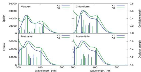
Fig. 10 The theoretical estimation of the vertical absorption spectrum for **K1** and **K2** obtained with the PBE0/6-311++G(d,p) approach in vacuum, chloroform, methanol and acetonitrile (PCM, linear response).
