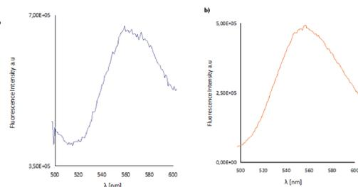
Fig. 15 Solid state emission spectra of (a) **K1\_2** material, (b) **K2\_2** material;  $\lambda_{\text{ex}} = 420 \text{ nm}$ ,  $\lambda_{\text{em}} = 554 \text{ nm}$  (**K1\_2**),  $\lambda_{\text{em}} = 565 \text{ nm}$  (**K2\_2**).
