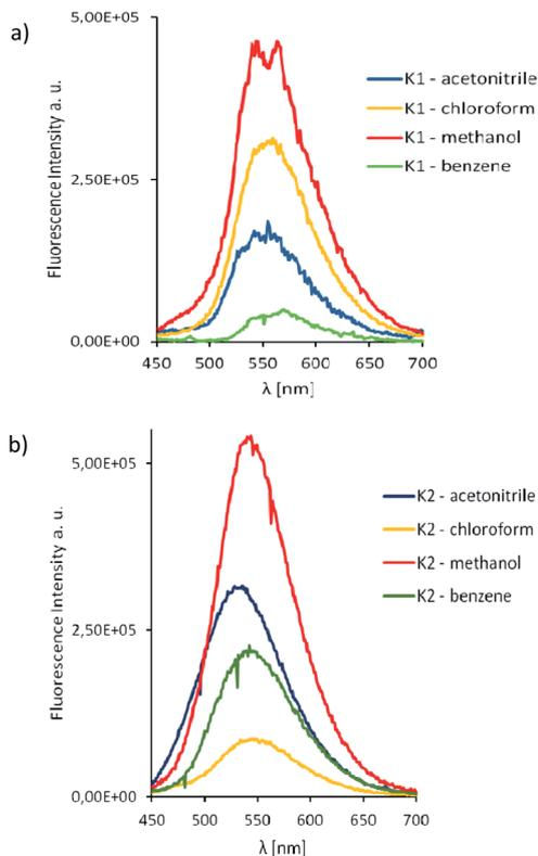
Fig. 11 Solution emission spectra of complexes **K1** and **K2**. (a) **K1** (b) **K2**  $\lambda_{\text{ex}} = 420$  nm (MeCN, chloroform, methanol and benzene  $1 \times 10^{-4}$  mol  $\text{dm}^{-3}$ , RT).
