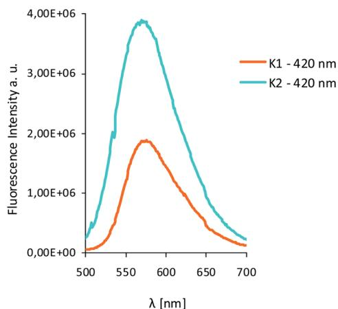
Fig. 12 Solid state emission spectra of complexes **K1** and **K2**  $\lambda_{\text{exc}}$  = 420 nm.
