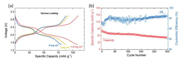
Fig. 5 (a) First galvanostatic discharge-charge profiles of EV-KB composite electrode at various mass loading at 0.2 mA cm<sup>-2</sup>. (b) Capacity retention and coulombic efficiency of EV-KB composite electrode of mass loading  $\sim$ 3 mg cm<sup>-2</sup> at 0.2 mA cm<sup>-2</sup>.
