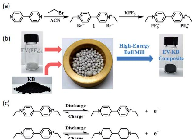
Fig. 1 (a) Schematic synthesis process of ethyl viologen dihexafluorophosphate (EV(PF<sub>6</sub>)<sub>2</sub>). (b) Schematic synthesis process of EV-KB composite. (c) Redox reaction mechanism of EV(PF<sub>6</sub>)<sub>2</sub>.
