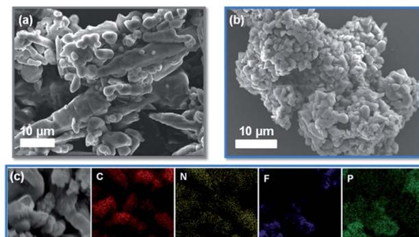
Fig. 2 SEM images of (a) EV(PF<sub>6</sub>)<sub>2</sub> and (b) EV-KB composite. (c) EDX images of EV-KB composite.
