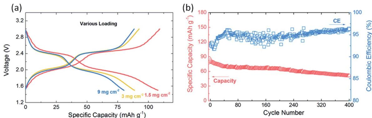
Fig. 5 (a) First galvanostatic discharge–charge profiles of EV-KB composite electrode at various mass loading at 0.2 mA cm<sup>-2</sup>. (b) Capacity retention and coulombic efficiency of EV-KB composite electrode of mass loading ~3 mg cm<sup>-2</sup> at 0.2 mA cm<sup>-2</sup>.
