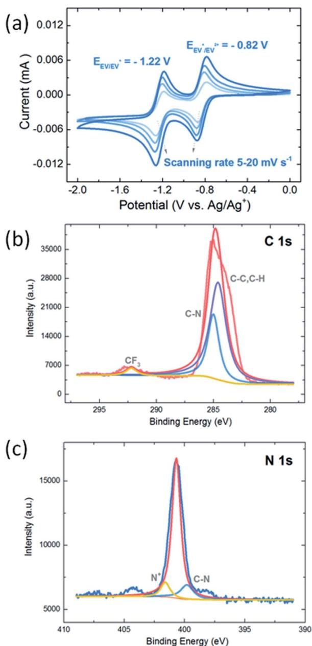
Fig. 3 (a) Cyclic voltammetry results of 2 mM EV(PF<sub>6</sub>)<sub>2</sub> in 1 M LiClO<sub>4</sub> in PC at various scanning rates. XPS spectra of EV(PF<sub>6</sub>)<sub>2</sub> in (b) C 1s and (c) N 1s regions.
