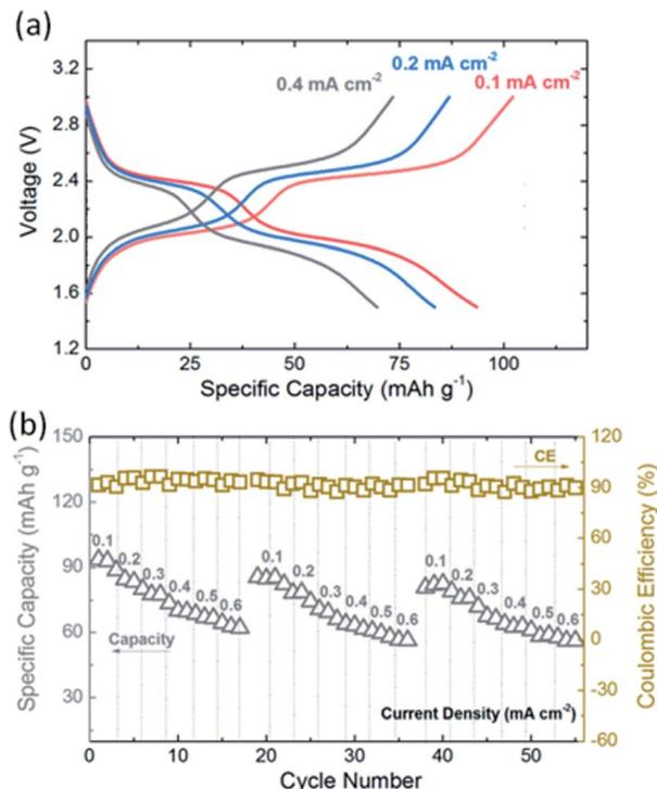
Fig. 4 (a) First galvanostatic discharge–charge profiles of EV-KB composite electrode between 0.1 and 0.4 mA cm<sup>-2</sup>. (b) Rate capability and coulombic efficiency of the EV-KB composite electrode at various current densities from 0.1 to 0.6 mA cm<sup>-2</sup>.
