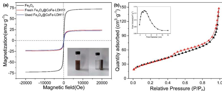
Fig. 3 The magnetic hysteresis loop of  $\text{Fe}_3\text{O}_4$ , fresh and used  $\text{Fe}_3\text{O}_4$ @CoFe-LDH11, the inset showed the separation of  $\text{Fe}_3\text{O}_4$ @CoFe-LDH11 from solution by external magnetic field (a) and  $\text{N}_2$  adsorption–desorption isotherms of  $\text{Fe}_3\text{O}_4$ @CoFe-LDH11 (b).
