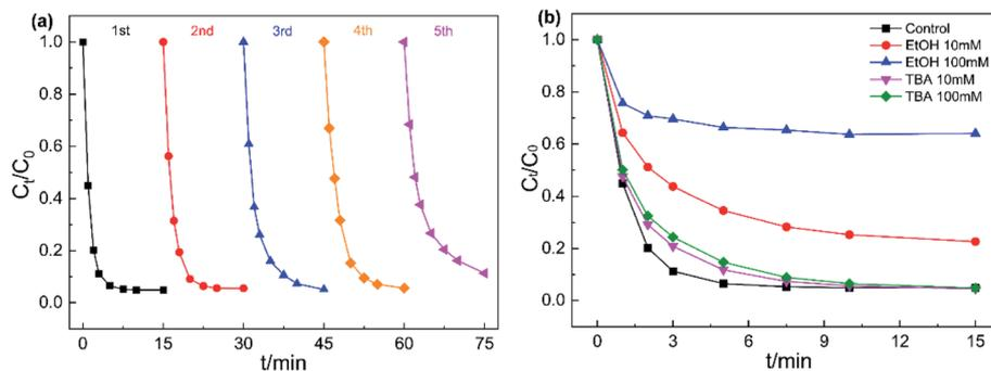
Fig. 8 Reusability of Fe<sub>3</sub>O<sub>4</sub>@CoFe-LDH for the degradation of AO7 (a), effect of TBA and EtOH on AO7 degradation (b). Experiment conditions: pH = 6,  $T = 298$  K,  $V = 0.1$  L, [AO7] = 40 mg L<sup>-1</sup>, [catalyst] = 50 mg L<sup>-1</sup>, [PMS] = 0.12 mM.
