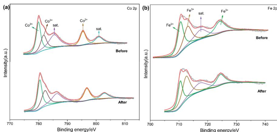
Fig. 9 XPS spectra of (a) Co 2p and (b) Fe 2p of fresh and used Fe<sub>3</sub>O<sub>4</sub>@CoFe-LDH.
