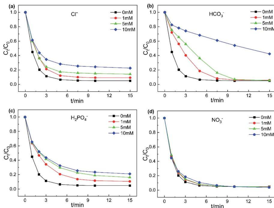
Fig. 7 Effects of anions on AO7 degradation (a)  $Cl^-$ , (b)  $HCO_3^-$ , (c)  $H_2PO_4^-$  and (d)  $NO_3^-$ . Experiment conditions: pH = 6,  $T = 298$  K,  $V = 0.1$  L,  $[AO7] = 40$  mg  $L^{-1}$ ,  $[catalyst] = 50$  mg  $L^{-1}$ ,  $[PMS] = 0.12$  mM.
