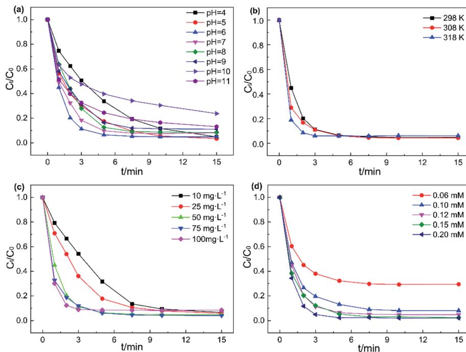
Fig. 6 Effects of (a) initial of pH, (b) temperature, (c) catalyst concentrations and (d) PMS dosages on AO7 removal efficiency. Experiment conditions: pH = 6 (except a),  $T = 298$  K (except b),  $V = 0.1$  L,  $[AO7] = 40$  mg  $L^{-1}$ ,  $[catalyst] = 50$  mg  $L^{-1}$  (except c),  $[PMS] = 0.12$  mM (except d).
