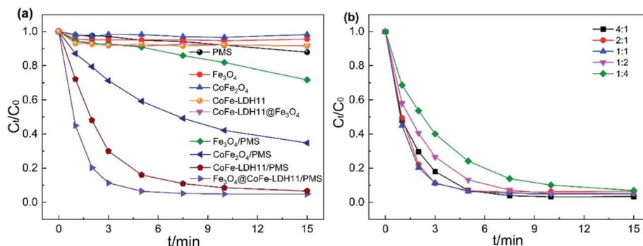
Fig. 5 AO7 degradation in different system (a) and effect of Co/Fe molar ratio on AO7 degradation (b). Experiment conditions: pH = 6,  $T = 298$  K,  $V = 0.1$  L,  $[AO7] = 40$  mg L<sup>-1</sup>,  $[catalyst] = 50$  mg L<sup>-1</sup>,  $[PMS] = 0.12$  mM.
