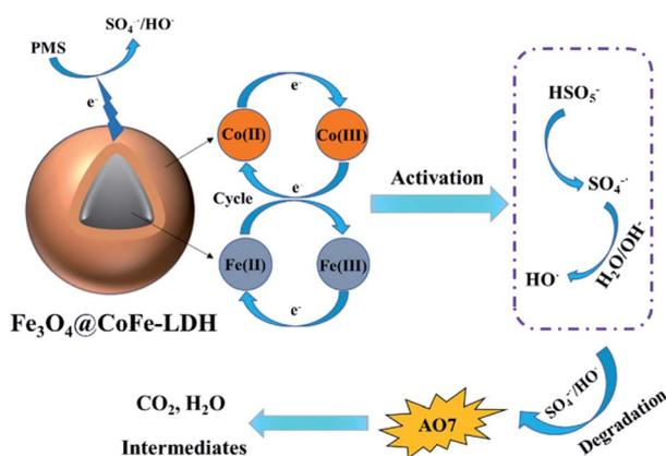
Fig. 10 The possible mechanisms of Fe<sub>3</sub>O<sub>4</sub>@CoFe-LDH activated PMS for AO7 degradation.
