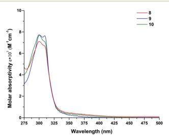
Fig. 6 UV-vis absorption spectra of 8–10 in EtOH (5  $\times$  10<sup>-5</sup> M)
