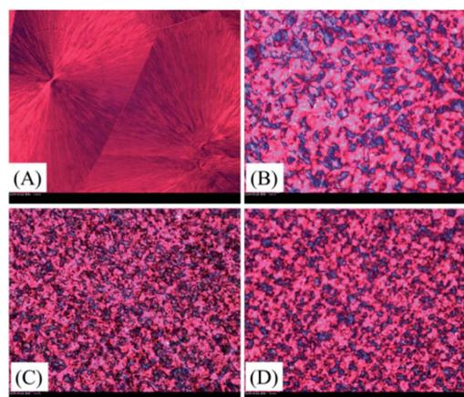
Fig. 5 Polarized optical microscopic images for spherulitic morphology of PLA (A), PLA/TEAP<sub>0.5</sub> (B), PLA/TEAP<sub>1.0</sub> (C), and PLA/TEAP<sub>3.0</sub> (D) isothermally crystallized at 125 °C after the sample films were prepared by casting and evaporation of 50 mg ml<sup>-1</sup> polymer chloroform solution on microscopic cover glass.
