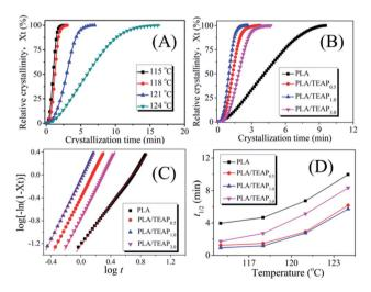
Fig. 4 Development of relative crystallinity with crystallization time at different crystallization temperatures for PLA/TEAP $_{1.0}$  (A); development of relative crystallinity with crystallization time at 115 °C for PLA and PLA/TEAP (B); Avrami plots of PLA and PLA/TEAP at 115 °C (C); crystallization temperature dependence of  $t_{1/2}$  for PLA and PLA/TEAP (D).
