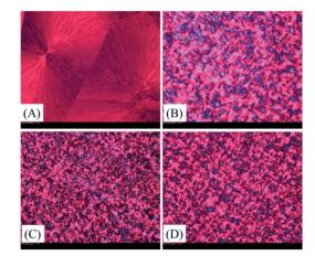
Fig. 5 Polarized optical microscopic images for spherulitic morphology of PLA (A), PLA/TEAP $_{0.5}$  (B), PLA/TEAP $_{1.0}$  (C), and PLA/TEAP $_{3.0}$  (D) isothermally crystallized at 125 °C after the sample films were prepared by casting and evaporation of 50 mg ml $^{-1}$  polymer chloroform solution on microscopic cover glass.
