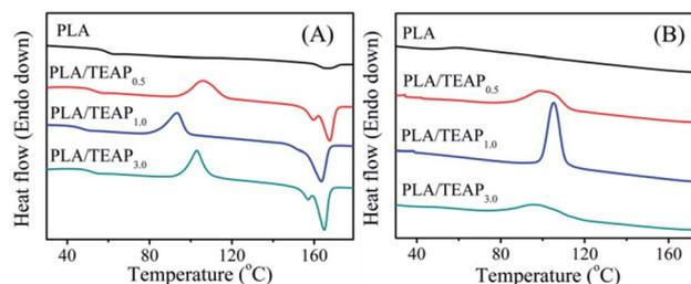
Fig. 3 DSC thermograms of samples, first heating scans from melt-quenched state at a rate of  $10\text{ }^\circ\text{C min}^{-1}$  (A); cooling scans at a rate of  $10\text{ }^\circ\text{C min}^{-1}$  (B).
