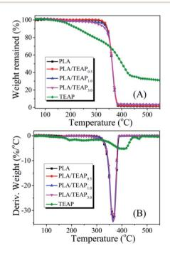
Fig. 2 TGA (A) and DTG (B) curves of PLA and PLA/TEAP under nitrogen atmosphere.
