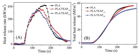
Fig. 7 The curves of heat release rate (A) and total heat release (B) versus time for PLA and PLA/TEAP
