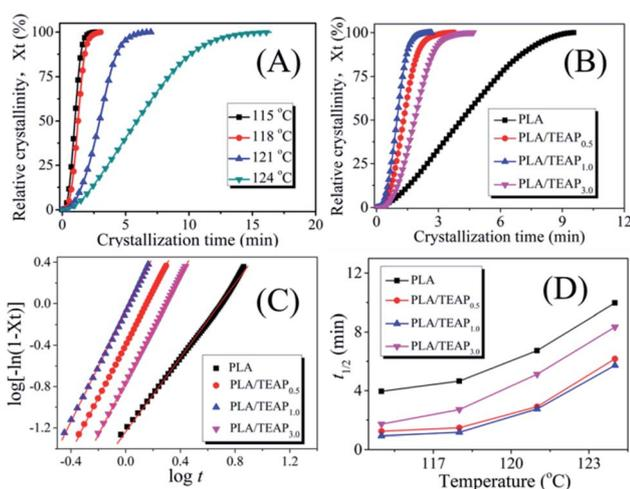
Fig. 4 Development of relative crystallinity with crystallization time at different crystallization temperatures for PLA/TEAP<sub>1.0</sub> (A); development of relative crystallinity with crystallization time at 115 °C for PLA and PLA/TEAP (B); Avrami plots of PLA and PLA/TEAP at 115 °C (C); crystallization temperature dependence of  $t_{1/2}$  for PLA and PLA/TEAP (D).
