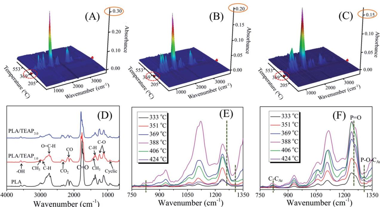
Fig. 8 The three-dimensional TG-FTIR spectra for the thermal decomposition of PLA (A), PLA/TEAP<sub>1.0</sub> (B) and PLA/TEAP<sub>3.0</sub> (C); the degraded volatiles of PLA and PLA/TEAP at 388 °C (D); the degraded volatiles of PLA (E) and PLA/TEAP<sub>3.0</sub> (F) at variable temperatures.
