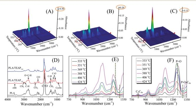
Fig. 8 The three-dimensional TG-FTIR spectra for the thermal decomposition of PLA (A), PLA/TEAP<sub>1.0</sub> (B) and PLA/TEAP<sub>3.0</sub> (C); the degraded volatiles of PLA and PLA/TEAP at 388 °C (D); the degraded volatiles of PLA (E) and PLA/TEAP<sub>3.0</sub> (F) at variable temperatures.
