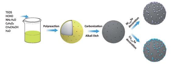
Fig. 1 The schematic of the preparation process of  $M_{0.85}$ Se-NHCS (M = Ni, Co).
