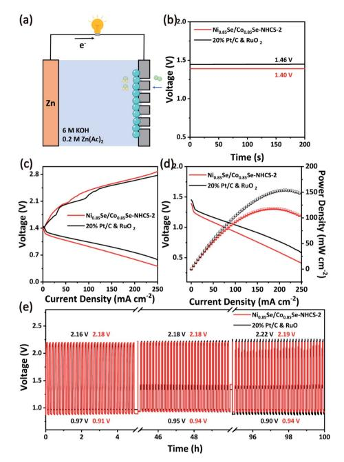
Fig. 7 (a) the schematic of the zinc–air battery. (b) The open-circuit curves, (c) charge and discharge polarization curves, (d) discharge polarization curves and corresponding the power density curves and the long-term stability by charge and discharge at 25 mA cm $^{-2}$  of zinc–air battery assemble with Ni<sub>0.85</sub>Se/Co<sub>0.85</sub>Se-NHCS-2 and 20% Pt/C $\theta$ RuO<sub>2</sub>.
