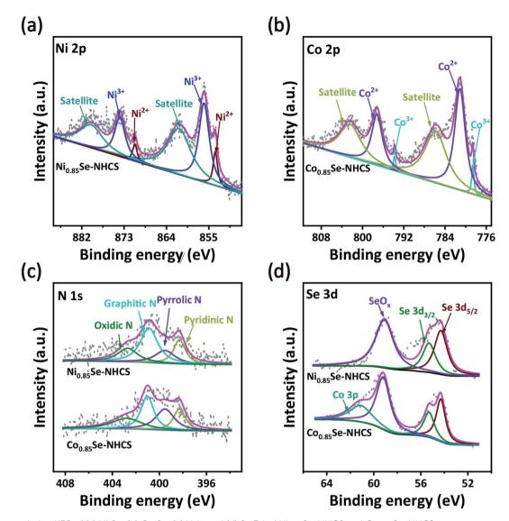
Fig. 4 High-resolution XPS of (a) Ni 2p, (b) Co 2p, (c) N 1s and (d) Se 3d of  $Ni_{0.85}$ Se-NHCS and  $Co_{0.85}$ Se-NHCS.
