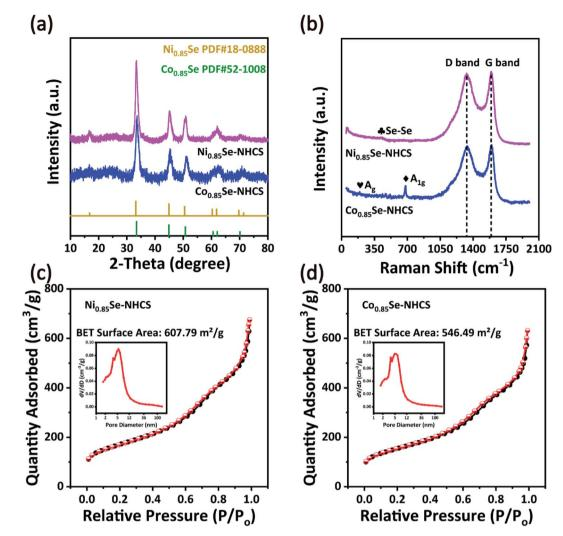
Fig. 3 (a) The XRD patterns and (b) Raman patterns of  $Ni_{0.85}$ Se-NHCS and  $Co_{0.85}$ Se-NHCS. (c)  $N_2$  adsorption/desorption isotherms of  $Ni_{0.85}$ Se-NHCS (inset: pore size distribution) and (d)  $N_2$  adsorption/desorption isotherms of  $Co_{0.85}$ Se-NHCS (inset: pore size distribution).
