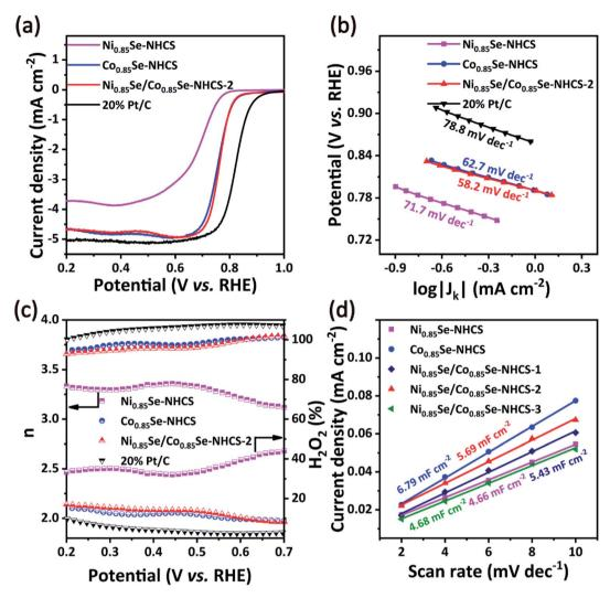
Fig. 5 (a) Linear sweep voltammogram curves for ORR and corresponding (b) Tafel curves, (c) converted electron transfer number and hydrogen peroxide yield of Ni<sub>0.85</sub>Se-NHCS, Ni<sub>0.85</sub>Se-NHCS, Co<sub>0.85</sub>Se/Ni<sub>0.85</sub>Se-NHCS-2, and 20% Pt/C. (d) The ECSA of synthesized samples by CV measurement in different scan rates.
