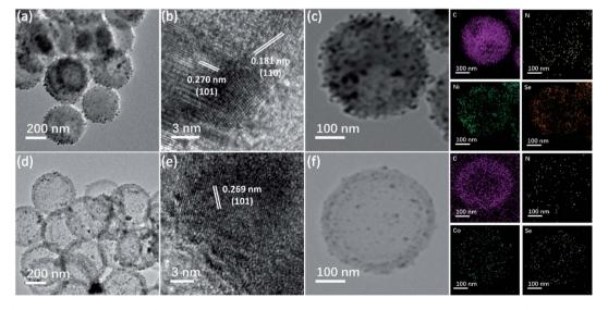
Fig. 2 (a and d) The TEM images, (b and e) high-resolution transmission electron microscopy image, and (c and f) EDX mappings of Ni<sub>0.85</sub>Se-NHCS and Co<sub>0.85</sub>Se-NHCS, respectively.
