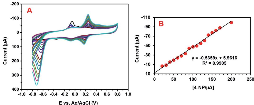
Fig. 9 (A) The obtained CV response for the GCE/CNF/CuCrO<sub>2</sub> electrode for the detection of 0.1 to  $200 \mu\text{M}$  4-NP in PBS. (B) Calibration plot between the peak current and concentration of 4-NP.
