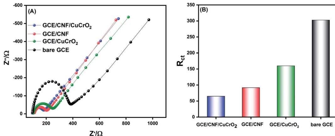
Fig. 7 (A) EIS studies of (a) bare GCE, (b) GCE/CNF, (c) GCE/CuCrO<sub>2</sub>, and (d) GCE/CNF/CuCrO<sub>2</sub> modified electrodes in 0.1 M KCl at 5 mM [Fe(CN)<sub>6</sub>]<sup>3-/4-</sup>. (B) R<sub>ct</sub> values of bare GCE, GCE/CuCrO<sub>2</sub>, GCE/CNF, and GCE/CNF/CuCrO<sub>2</sub> electrodes.
