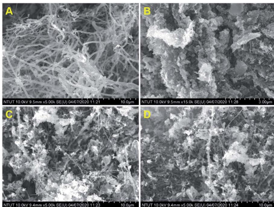
Fig. 2 SEM image of (A) CNF, (B)  $\text{CuCrO}_2$ , (C and D) CNF/ $\text{CuCrO}_2$ .
