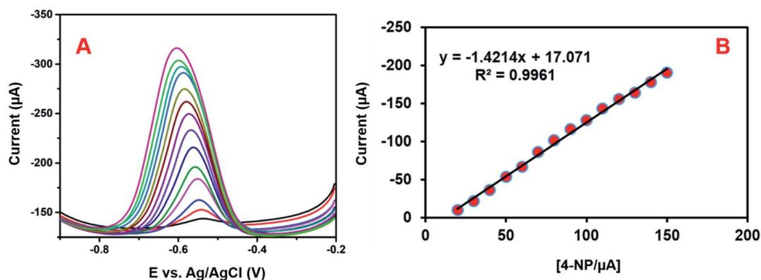
Fig. 12 (A) DPV performance of GCE/CNF/CuCrO<sub>2</sub> electrode in 4-NP solution at different concentrations. (B) Plot of peak current versus concentration of 4-NP.
