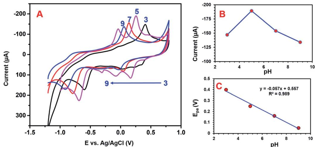
Fig. 10 (A) Cyclic voltammogram of GCE/CNF/CuCrO<sub>2</sub> electrode under deoxygenated conditions at pH 3 to pH 9. (B) The inset shows the pH values versus peak current. (C) The inset shows the pH values versus oxidation peak potential.
