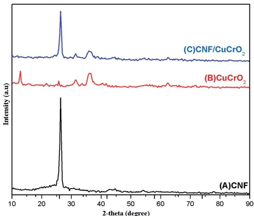
Fig. 1 XRD spectra of (A) CNF, (B) CuCrO<sub>2</sub>, and (C) CNF/CuCrO<sub>2</sub> powder.
