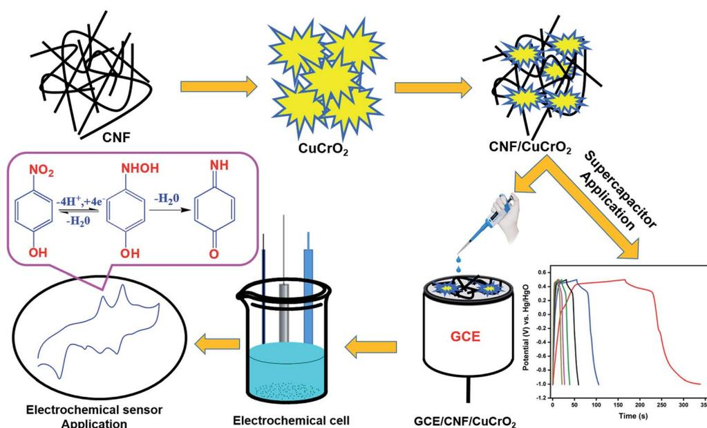
Scheme 1 Preparation of GCE/CNF/CuCrO<sub>2</sub> electrode for detection of 4-NP and supercapacitor.
