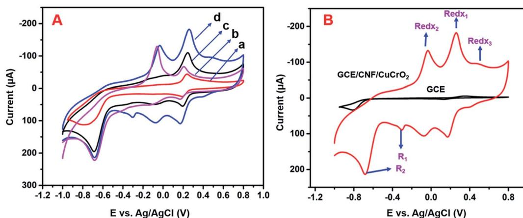
Fig. 8 (A) CV studies of (a) bare GCE, (b) GCE/CNF, (c) GCE/CuCrO<sub>2</sub>, and (d) GCE/CNF/CuCrO<sub>2</sub> electrodes in the presence of 1.0 μM of 4-NP in PBS (pH = 5.0) at a scan rate of 50 mV s<sup>-1</sup> and (B) CV response of (a) GCE/CNF/CuCrO<sub>2</sub> and (b) bare GCE in the presence of 4-NP in PBS (pH = 5.0).
