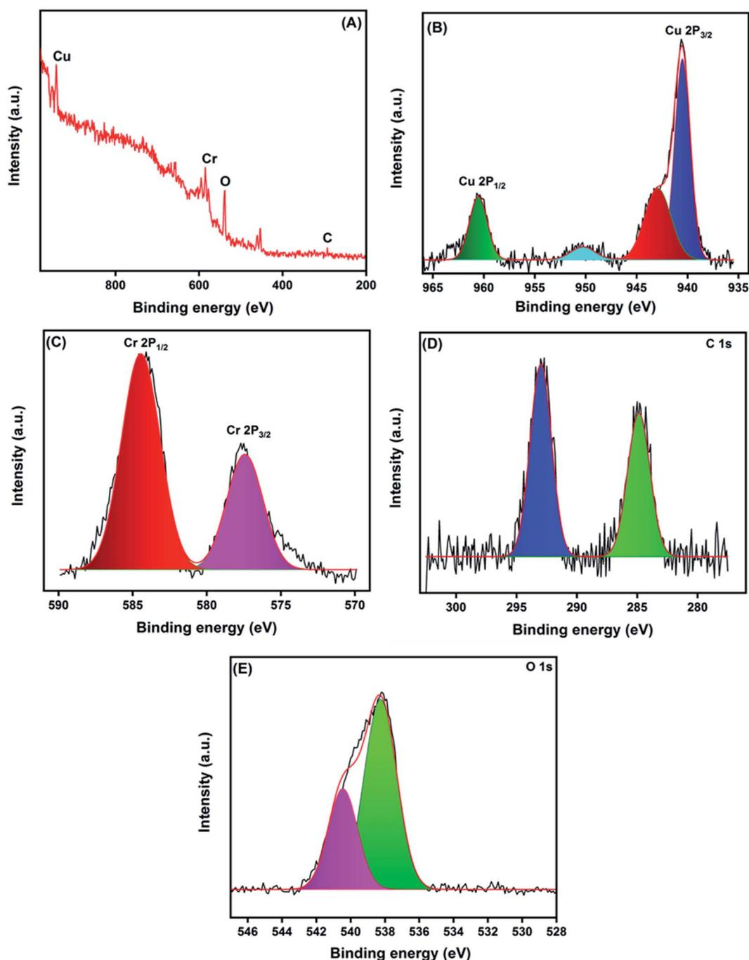
Fig. 6 XPS survey spectrum of CNF/CuCrO<sub>2</sub> composite (A), core level spectrum of Cu 2p (B), Cr 2p (C), C 1s (D), and O 1s (E).
