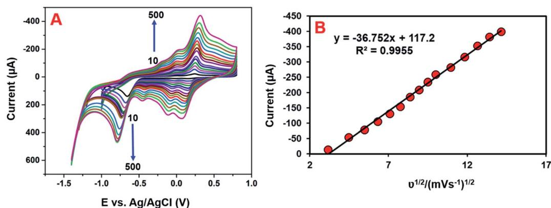
Fig. 11 (A) CV curves of GCE/CNF/CuCrO<sub>2</sub> electrode in the presence of 1.0  $\mu\text{M}$  4-NP in 0.05 M PBS (pH 5.0) were observed at various scan rates of 10–500  $\text{mV s}^{-1}$ . (B) Correlations between the peak currents and the square root of the scan rate.
