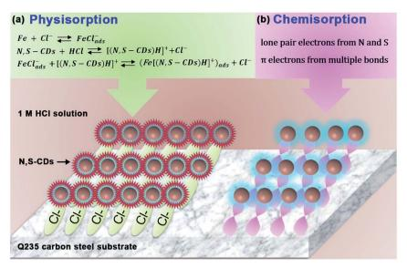
Fig. 13 Inhibition mechanism of N,S-CDs on the Q235 carbon steel surface in 1 M HCl solution
