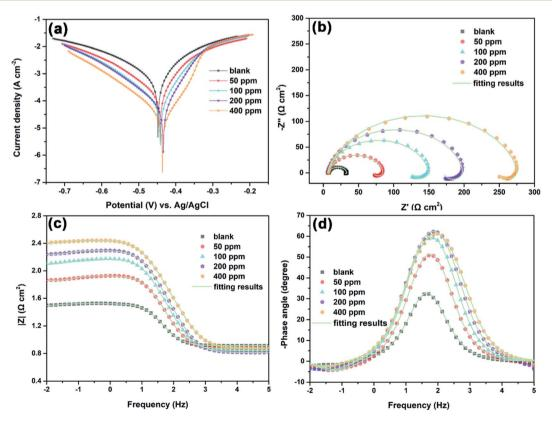
Fig. 3 (a) Polarization and (b-d) EIS curves of Q235 carbon steel in 1 M HCl solution with and without different concentrations of N,S-CDs at room temperature.
