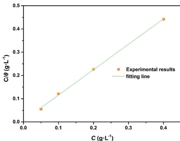
**Fig. 8** Langmuir adsorption isotherm ( $\frac{C_{inh}}{\theta}$  versus  $C_{inh}$ ) of N,S-CDs in 1 M HCl at room temperature.
