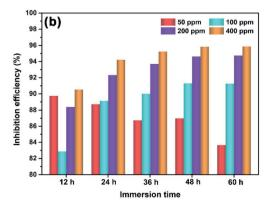
Fig. 5 (a) Corrosion rate and (b) inhibition efficiency for Q235 carbon steel during 60 h of immersion in 1 M HCl without and with different concentrations of N.S-CDs
