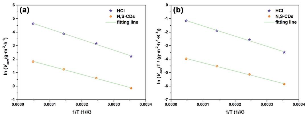
**Fig. 9** (a) Arrhenius plots and (b) plots of  $\ln V_{corr}/T$  versus  $1/T$  for the corrosion of Q235 carbon steel in 1 M HCl with 400 ppm N,S-CDs.
