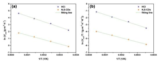
(a) Arrhenius plots and (b) plots of  $\ln V_{corr}/T$  versus 1/T for the corrosion of Q235 carbon steel in 1 M HCl with 400 ppm N,S-CDs.
