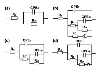
Fig. 7 Equivalent circuits used for fitting EIS data at different immersion time points, (a) 24 h in blank solution, (b) 6 h, (c) 12 h, and (d) 24 h in 400 ppm N.S-CDs.
