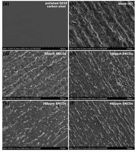
Fig. 10 SEM images of Q235 carbon steel before and after 60 h of immersion in 1 M HCl solution with and without different concentrations of N,S-CDs (a) polished Q235 carbon steel, (b) in blank HCl solution, and 1 M HCl solution with (c) 50 ppm, (d) 100 ppm, (e) 200 ppm and (f) 400 ppm of N,S-CDs.
