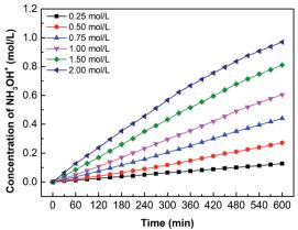
Fig. 12 The curves of hydroxylamine concentration over time for various oxime concentration ( $C_{\text{oxime}}=0.25 \text{ mol L}^{-1}$ , 0.50 mol L<sup>-1</sup>, 0.75 mol L<sup>-1</sup>, 1.00 mol L<sup>-1</sup>, 1.50 mol L<sup>-1</sup>, and 2.00 mol L<sup>-1</sup>).  $i=4.69\times10^{-2} \text{ A cm}^{-2}$ .
