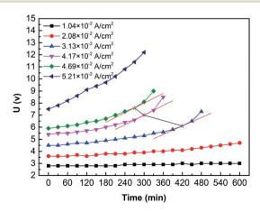
Fig. 11 The curves of the cell voltage over time under various current densities ( $i=1.04\times10^{-2}~{\rm A~cm^{-2}}$ ,  $2.08\times10^{-2}~{\rm A~cm^{-2}}$ ,  $3.13\times10^{-2}~{\rm A~cm^{-2}}$ ,  $4.17\times10^{-2}~{\rm A~cm^{-2}}$ ,  $4.69\times10^{-2}~{\rm A~cm^{-2}}$ , and  $5.21\times10^{-2}~{\rm A~cm^{-2}}$ ).  $C_{\rm oxime}=1.00~{\rm mol~L^{-1}}$ .
