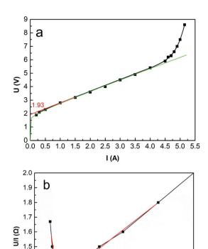
Fig. 5 (a) Initial cell voltage versus current intensity.  $C_{\text{oxime}} =$ 1.00 mol L<sup>-1</sup>, mass velocity = 135.0 g min<sup>-1</sup>, T = 25 °C. (b) R - 1/I
