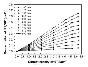
Fig. 7 The effect of current density on the hydroxylamine concentration.  $C_{\rm oxime}=1.00~{\rm mol}~{\rm L}^{-1}.$
