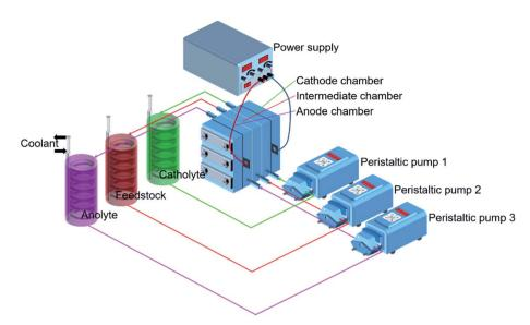
Fig. 3 Experiment equipment of the coupling process.
