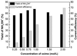
Fig. 10 The effect of oxime concentration on the yield of hydroxylaminea and current efficiency.  $i = 4.69 \times 10^{-2}$  A cm<sup>-2</sup>, time = 600 min, and concentration of H<sub>2</sub>SO<sub>4</sub> equals 1.00 mol L<sup>-1</sup>.
