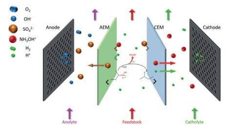
Fig. 2 The hydrolysis-electrodialysis coupling process.
