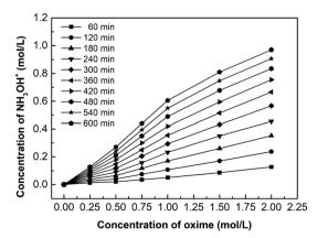
Fig. 9 The effect of oxime concentration on the hydroxylamine concentration.  $i=4.69\times 10^{-2}$  A cm<sup>-2</sup>.
