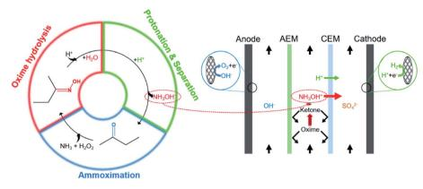
Fig. 4 Steps of the coupling process in the ED stack.
