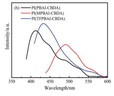
Fig. 7 Excitation-emission spectra of polyimide films based on dianhydride CBDA (a) excitation spectra, (b) emission spectra.
