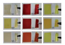
Fig. 5 Images of triphenyl imidazole-containing polyimide films (a) PI(PBAI-CBDA), (b) PI(PBAI-PMDA), (c) PI(PBAI-6FDA), (d) PI(MPBAI-CBDA), (e) PI(MPBAI-PMDA), (f) PI(MPBAI-6FDA), (g) PI(TFPBAI-CBDA), (h) PI(TFPBAI-PMDA), (i) PI(TFPBAI-6FDA).
