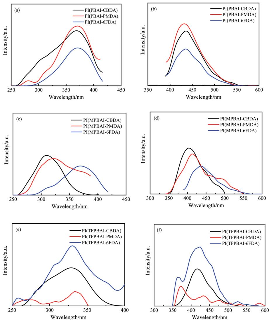
Fig. 12 Excitation–emission spectra of polyimide solution in DMAC ( $1 \times 10^{-4} \text{ g L}^{-1}$ ) (a) excitation spectra of PIs with PBAI, (b) emission spectra of PIs with PBAI, (c) excitation spectra of PIs with MPBAI (d) emission spectra of PIs with MPBAI, (e) excitation spectra of PIs with TFPBAI, (f) emission spectra of PIs with TFPBAI.
