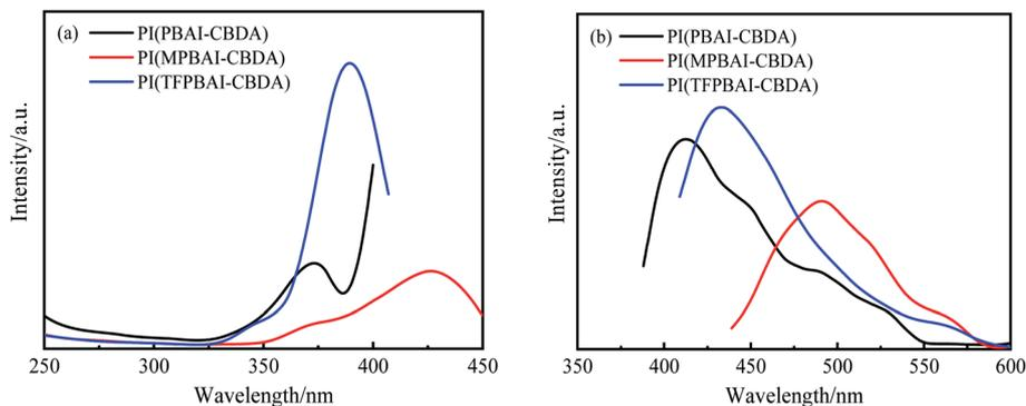
Fig. 7 Excitation–emission spectra of polyimide films based on dianhydride CBDA (a) excitation spectra, (b) emission spectra.
