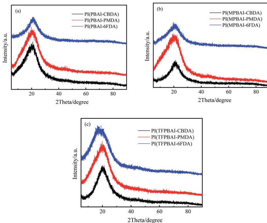
Fig. 2 XRD patterns of triphenyl imidazole-containing polyimides (a) PIs based on PBAI, (b) PIs based on MPBAI, (c) PIs based on TFPBAI.
