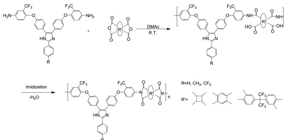
Scheme 2 Synthesis of triphenyl imidazole-containing polyimides.
