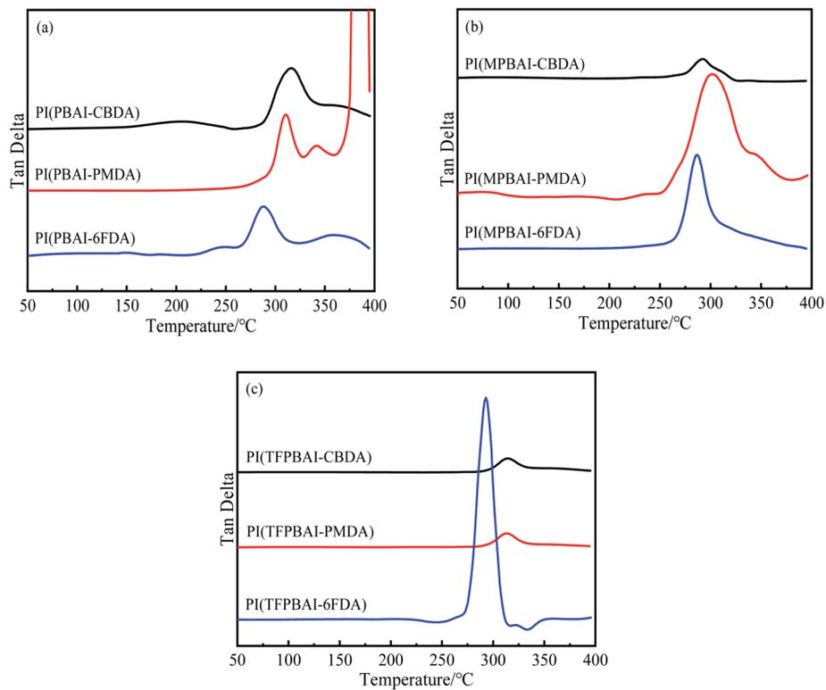
Fig. 3 Tan  $\delta$ - $T$  curves of triphenyl imidazole-containing polyimides (a) Pls based on PBAI, (b) Pls based on MPBAI, (c) Pls based on TFPBAI.
