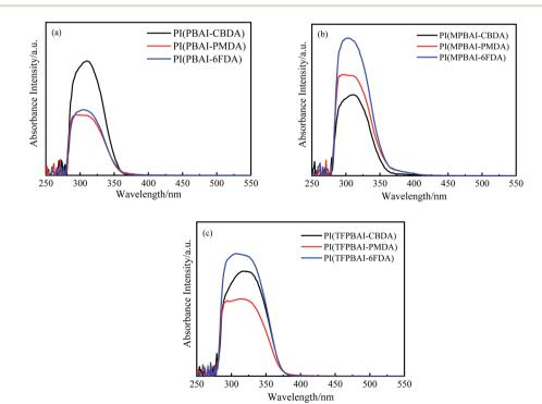
Fig. 11 Ultraviolet absorbance spectra of polyimides solution in DMAc (a) PIs based on PBAI, (b) PIs based on MPBAI, (c) PIs based on TFPBAI.
