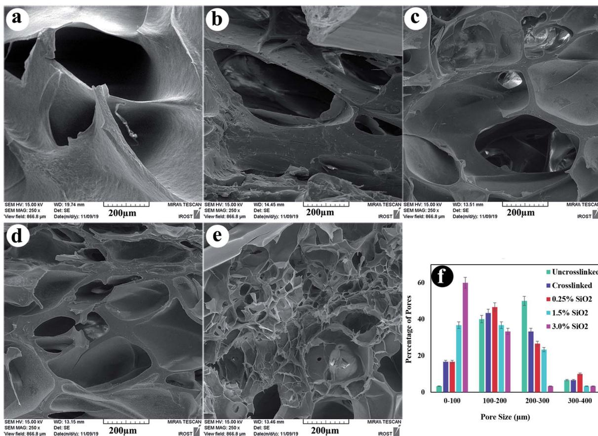
**Fig. 4** Cross-section morphology of freeze-dried hydrogels (a) uncrosslinked, (b) crosslinked, (c) containing 0.25% SiO<sub>2</sub>, (d) 1.5% SiO<sub>2</sub>, (e) 3.0% SiO<sub>2</sub>, and (f) pore size distribution of the samples.
