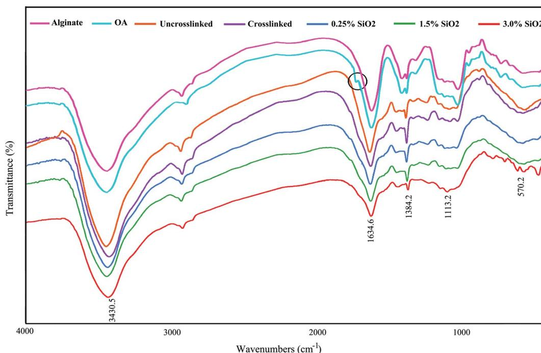
Fig. 1 FTIR spectrum of alginate, oxidized alginate, and the hydrogels.
