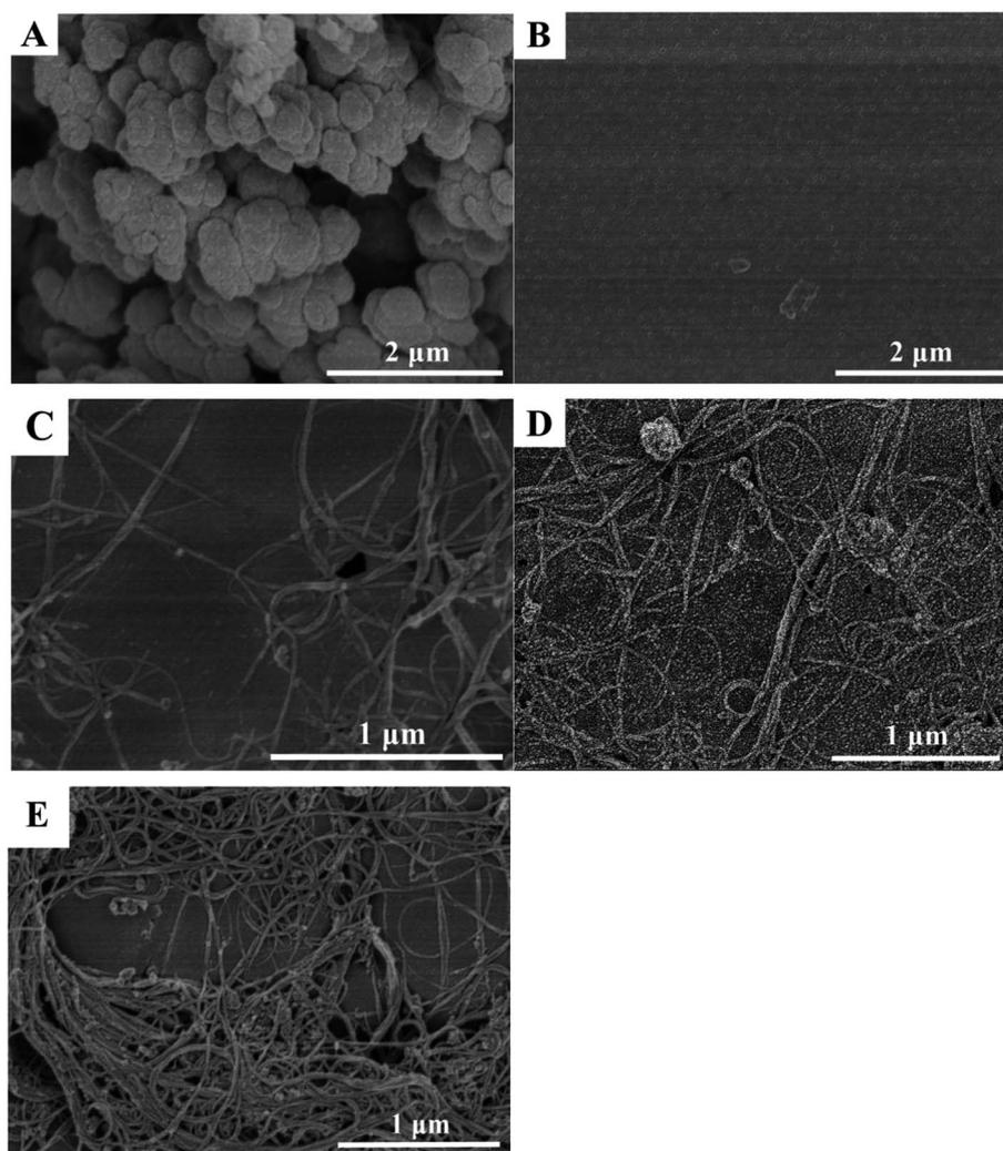
Fig. 2 FE-SEM images of the prepared samples: *in situ* polymerized PPy powder (A); interfacial polymerized PPy film (B); interfacial polymerized PPy/SWCNTs (0.3 mg) composite film (C); interfacial polymerized PPy/SWCNTs (0.5 mg) composite film (D); interfacial polymerized PPy/SWCNTs (0.8 mg) composite film (E).
