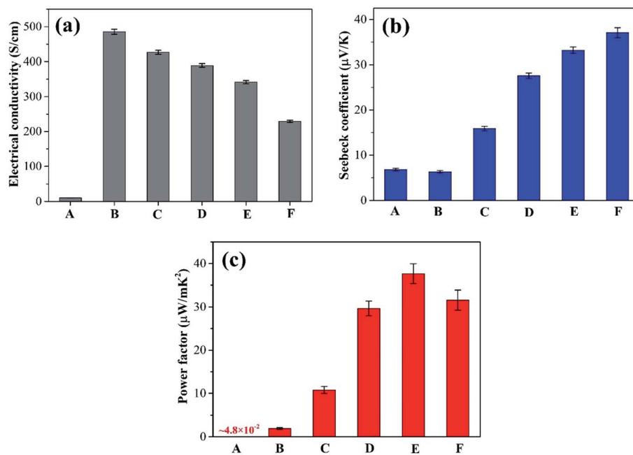
Fig. 5 Electrical conductivity (a), Seebeck coefficient (b) and power factor (c) of the prepared samples: *in situ* polymerized PPy powder (A); interfacial polymerized PPy film (B); interfacial polymerized PPy/SWCNTs (0.3 mg) composite film (C); interfacial polymerized PPy/SWCNTs (0.5 mg) composite film (D); interfacial polymerized PPy/SWCNTs (0.8 mg) composite film (E); interfacial polymerized PPy/SWCNTs (1 mg) composite film (F).
