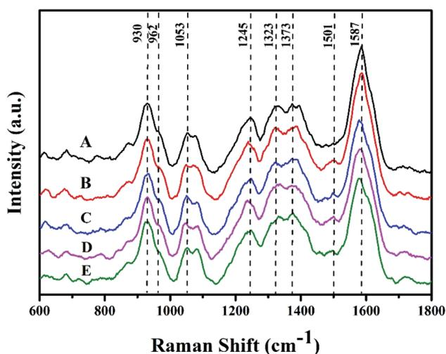
Fig. 4 Raman spectra of the prepared samples: *in situ* polymerized PPY powder (A); interfacial polymerized PPY film (B); interfacial polymerized PPY/SWCNTs (0.3 mg) composite film (C); interfacial polymerized PPY/SWCNTs (0.5 mg) composite film (D); interfacial polymerized PPY/SWCNTs (0.8 mg) composite film (E).
