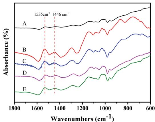
Fig. 3 FTIR spectra of the prepared samples: *in situ* polymerized PPY powder (A); interfacial polymerized PPY film (B); interfacial polymerized PPY/SWCNTs (0.3 mg) composite film (C); interfacial polymerized PPY/SWCNTs (0.5 mg) composite film (D); interfacial polymerized PPY/SWCNTs (0.8 mg) composite film (E).
