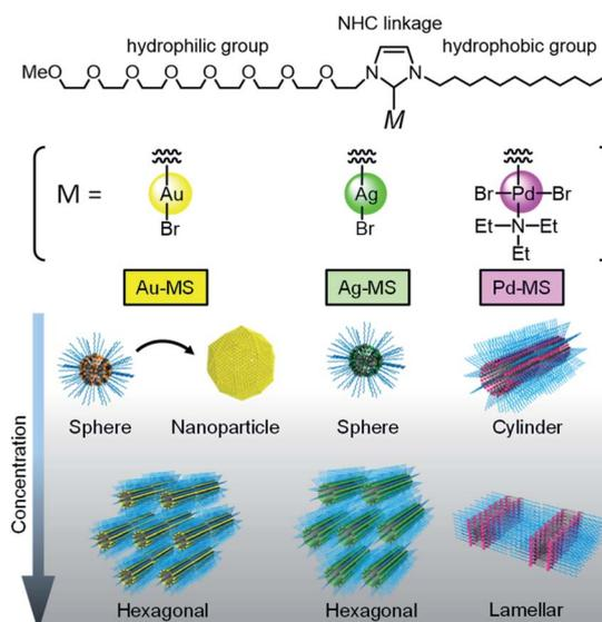
Fig. 1 Metallosurfactants (MSs) and their self-assembled structures.
