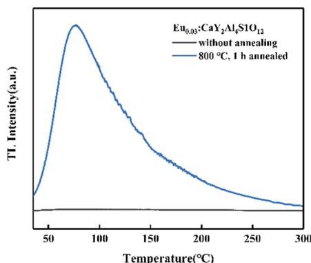
Fig. 14 TL spectrum of the R800 sample.
