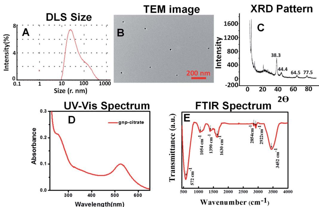
Fig. 1 (A) DLS size (B) TEM image (C) XRD pattern (D) UV-Vis spectrum ( $328\text{ g mL}^{-1}$  aqueous solution) (E) FTIR spectrum of gnp-citrate.
