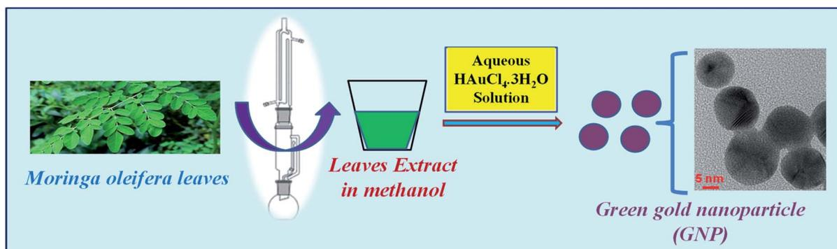
Scheme 1 A pictorial representation of the preparation of *M. oleifera* leaves extract in methanol followed by synthesis of green gold nanoparticles, reduced and stabilized by methanolic extract of *M. oleifera* leaves.
