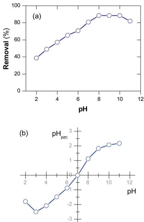
Fig. 8 (a) Effect of pH on MB adsorption efficiency and (b) pH at point of zero charge of D-FA (initial MB concentration = 30 g L<sup>-1</sup>).
