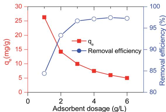
Fig. 9 Effect of adsorbent dosage on MB adsorption capacity and removal efficiency of D-FA (initial MB concentration = 30 g L<sup>-1</sup>).
