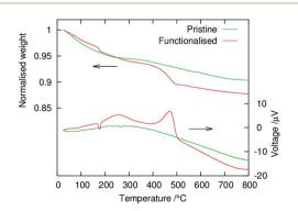
Fig. 4 TG-DTA curves of the pristine and surface-functionalised  $MgMn_2O_4$  powders.
