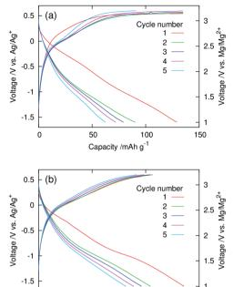
Fig. 5 Galvanostatic charge–discharge curves of dry composite cathodes of the (a) pristine and (b) surface–functionalised MgMn $_2$ O $_4$  prepared with the active material : AB : PTFE ratio of 60 : 30 : 10 (wt%) and recorded using a three-electrode setup at 100 °C.
