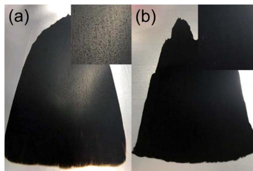
Fig. 6 Photographs of composite slurry-coated cathodes of the (a) pristine and (b) surface-functionalised  $\text{MgMn}_2\text{O}_4$  applied on Al foil, prepared with the active material : CNT : PVDF ratio of 93 : 4 : 3 (wt%). The widths of the coated area are  $\sim 10 \text{ cm}$ . The top-right inset in each figure shows  $\times 2$  magnified image of the coated area.
