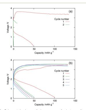
Fig. 9 Galvanostatic charge–discharge curves of coin-type cells with the composite slurry-coated cathodes of the (a) pristine and (b) surface–functionalised MgMn<sub>2</sub>O<sub>4</sub> shown in Fig. 6 and Mg–Al–Zn alloy anode recorded at 25  $^{\circ}$ C.
