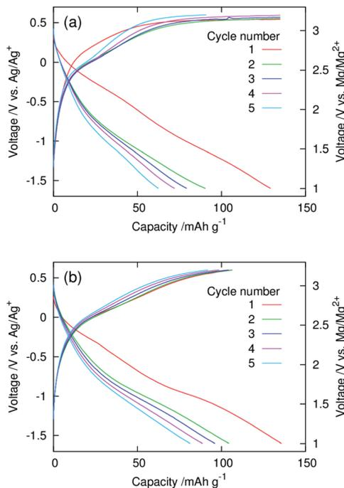
Fig. 5 Galvanostatic charge–discharge curves of dry composite cathodes of the (a) pristine and (b) surface-functionalised  $\text{MgMn}_2\text{O}_4$  prepared with the active material : AB : PTFE ratio of 60 : 30 : 10 (wt%) and recorded using a three-electrode setup at 100 °C.
