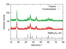
Fig. 1 Powder XRD patterns of the pristine and surface-functionalised  $MgMn_2O_4$  powders. Simulated pattern was calculated using RIETAN-FP<sup>40</sup> and the structural parameters of  $MgMn_2O_4$  reported in ref. 41.
