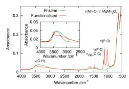
Fig. 2 ATR-FT-IR spectra of the pristine and surface-functionalised  $MgMn_2O_4$  powders. The inset shows magnified spectra and absorption spectrum of water (dashed line) taken from ref. 46.
