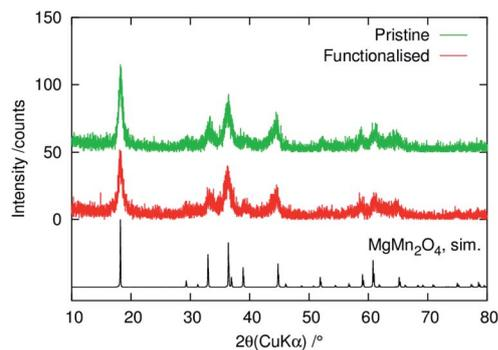
Fig. 1 Powder XRD patterns of the pristine and surface-functionalised  $\text{MgMn}_2\text{O}_4$  powders. Simulated pattern was calculated using RIETAN-FP<sup>40</sup> and the structural parameters of  $\text{MgMn}_2\text{O}_4$  reported in ref. 41.
