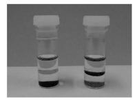
Fig. 3 Pristine (left) and surface-functionalised (right) MgMn $_2$ O $_4$  powders dispersed in a biphasic mixture of water (bottom layer) and toluene (top layer).
