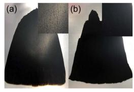
Fig. 6 Photographs of composite slurry-coated cathodes of the (a) pristine and (b) surface-functionalised MgMn<sub>2</sub>O<sub>4</sub> applied on Al foil, prepared with the active material: CNT: PVDF ratio of 93: 4: 3 (wt%). The widths of the coated area are  $\sim$ 10 cm. The top-right inset in each figure shows  $\times$ 2 magnified image of the coated area.
