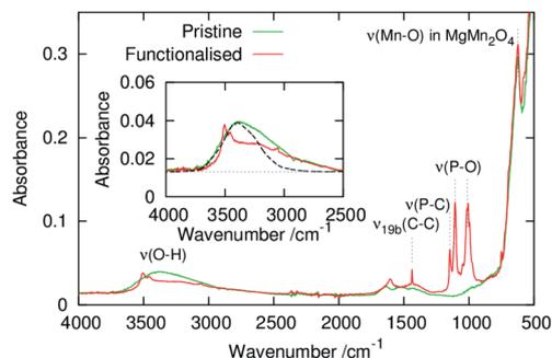
Fig. 2 ATR-FT-IR spectra of the pristine and surface-functionalised  $\text{MgMn}_2\text{O}_4$  powders. The inset shows magnified spectra and absorption spectrum of water (dashed line) taken from ref. 46.
