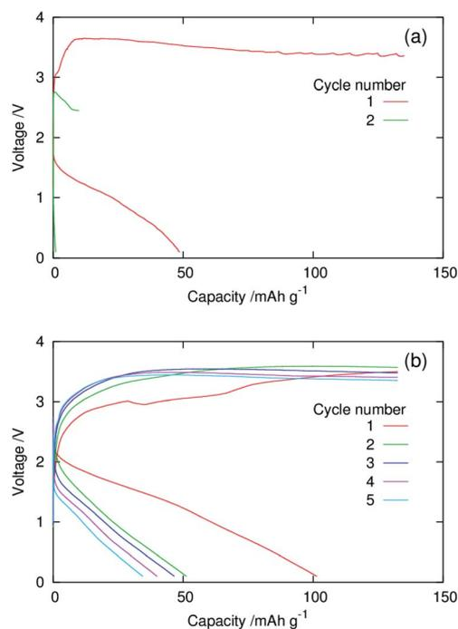
Fig. 9 Galvanostatic charge–discharge curves of coin-type cells with the composite slurry-coated cathodes of the (a) pristine and (b) surface-functionalised  $\text{MgMn}_2\text{O}_4$  shown in Fig. 6 and Mg–Al–Zn alloy anode recorded at  $25^\circ\text{C}$ .
