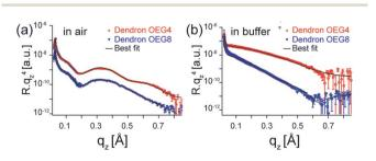
Fig. 2 High energy specular X-ray reflectivity (symbols) and best-fit results (lines) of dendron OEG4 (red) and dendron OEG8 (blue) measured (a) in air and (b) in buffer. The data collected in air are fitted with slab models, while those measured in buffer with diffusive interface models (eqn (1)). The structural parameters corresponding to the fits are presented in Tables 1 and 2, confirming the formation of monolayers.
