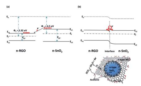
Fig. 4 Energy band diagram of RGO/SnO<sub>2</sub> (a) before and (b) after gas infusion reproduced from ref. 67 with permission from American Chemical Society, Copyright 2021.
