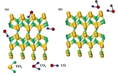
Fig. 2 (a) Ionized oxygen ions adsorbed on the surface of the sensing film and (b) CO vapor interacts with ionized oxygen ions giving back electrons to SMOs.
