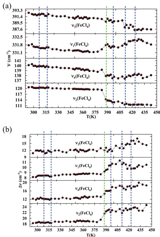
Fig. 8 (a) Raman wavenumbers of the inorganic part *versus* temperature. (DSC transitions in blue vertical lines. The green line shows a Raman transition which is not detected by the DSC). (b) Half widths of the Raman bands associated with [FeCl<sub>4</sub>]<sup>-</sup> *versus* temperature. (DSC transitions in blue vertical lines. The green line shows a Raman transition which is not detected by the DSC).
