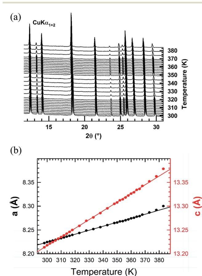
Fig. 5 (a) XRPD patterns collected upon heating in air from RT to 383 K after *in situ* dehydrating the  $[(C_2H_5)_4N]FeCl_4$  compound at 373 K. (b) Thermal evolutions of the hexagonal cell parameters *a* and *c* of the  $[(C_2H_5)_4N]FeCl_4$  compound determined from the refinement of the XRPD patterns by the Le Bail method.
