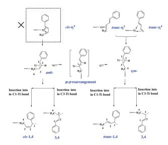
The suggested mechanism for polymerization of PBD
