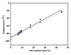
Fig. 5 Dependence of  $T_g$  of BD/PBD copolymers on the PBD incorporation content (mol%) ( $\blacksquare$ : experimental  $T_{g}$ ,  $\Delta$ : theoretical  $T_g$ ).
