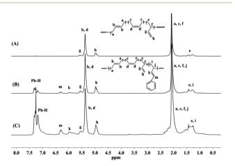
Fig. 1 Typical <sup>1</sup>H NMR spectra of polybutadiene and BD/PBD copolymers (A): polybutadiene; (B): BD/PBD copolymer with 7.84 mol% PBD (Table 1, run 3); (C): BD/PBD copolymer with 25.9 mol% PBD (Table 1, run 8).
