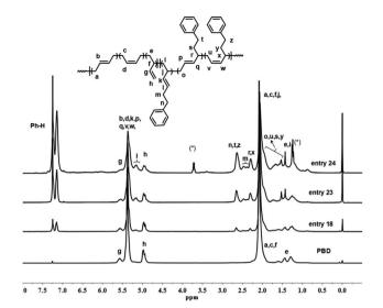
Fig. 7 <sup>1</sup>H NMR spectrum of BD/PEBD copolymer.
