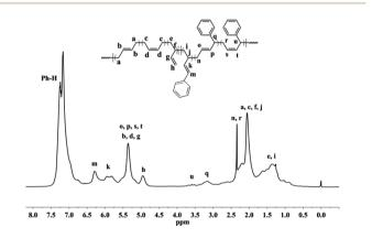
Fig. 3  $\,^{1}\mathrm{H}$  NMR spectrum of BD/PBD copolymer with 44.6 mol% PBD (Table 1, run 9).
