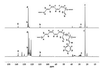
Fig. 2 Typical <sup>13</sup>C NMR spectra of polybutadiene and BD/PBD copolymers (A): polybutadiene; (B): BD/PBD copolymer with 25.9 mol% PBD (Table 1, run 8).
