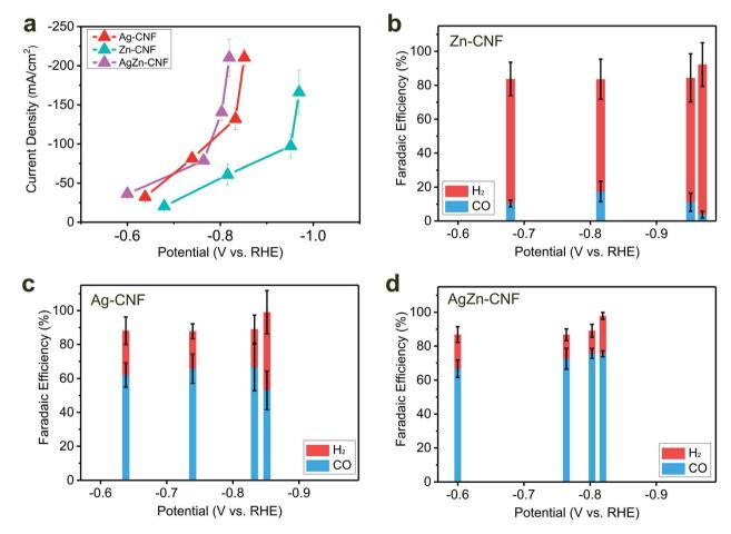
Fig. 4 (a) Current density *versus* applied potential of Zn–CNF, Ag–CNF and AgZn–CNF and the faradaic efficiency of electrocatalytic CO<sub>2</sub> reduction of (b) Zn–CNF, (c) Ag–CNF, and (d) AgZn–CNF.
