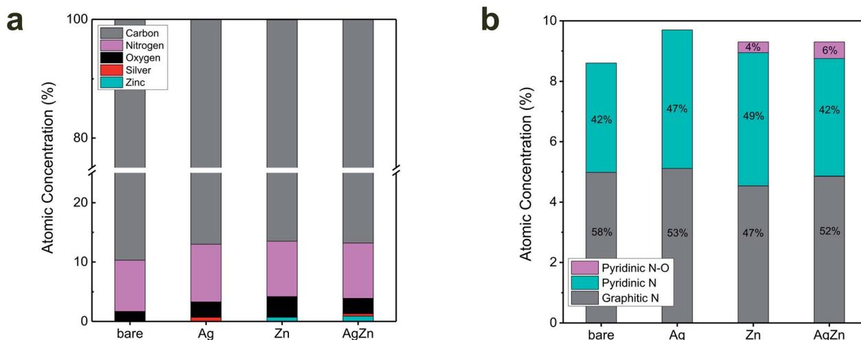
Fig. 3 XPS analysis of bare CNF, Ag-CNF, Zn-CNF and AgZn-CNF: (a) atomic concentration of each element and (b) deconvoluted N 1s results.
