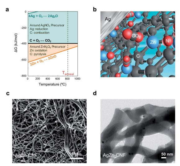
Fig. 1 Graphical image of the fabricated catalyst. (a) Ellingham diagram for thermodynamically designed calcination and (b) 3D atomic illustration of the local  $CO_2$  concentration between the Ag nanoparticles and single-atom Zn in the C matrix. (c) FESEM images of AgZn-CNF and (d) TEM images of AgZn-CNF.
