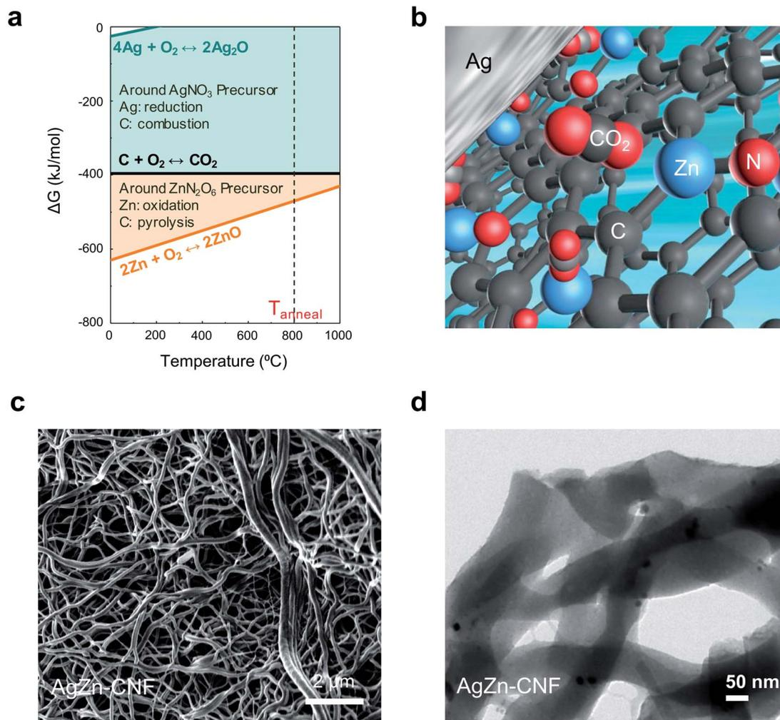
Fig. 1 Graphical image of the fabricated catalyst. (a) Ellingham diagram for thermodynamically designed calcination and (b) 3D atomic illustration of the local  $\text{CO}_2$  concentration between the Ag nanoparticles and single-atom Zn in the C matrix. (c) FESEM images of AgZn-CNF and (d) TEM images of AgZn-CNF.
