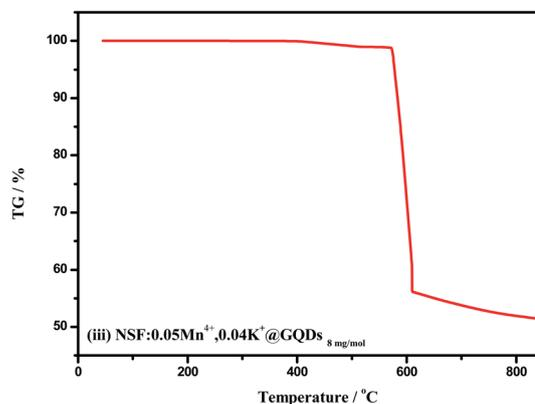
Fig. 6 TG of sample (iii) (NSF:0.05Mn<sup>4+</sup>,0.04K<sup>+</sup>@GQDs<sub>8 mg mol<sup>-1</sup></sub>).
