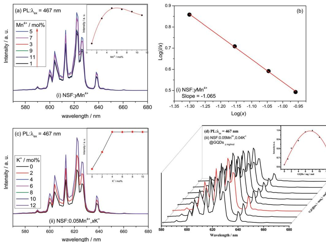
Fig. 4 Luminescent properties of NSF:yMn<sup>4+</sup>, NSF:0.05Mn<sup>4+</sup>,xK<sup>+</sup> and NSF:0.05Mn<sup>4+</sup>,0.04K<sup>+</sup>@GQDs<sub>8</sub> mg mol<sup>-1</sup>: (a), (c) and (d) PL spectra and (b) related line type of multipolar interaction.
