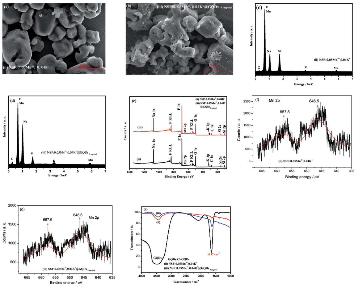
Fig. 2 SEM images, EDS, XPS and FTIR spectra of two samples, (ii) NSF:0.05Mn<sup>4+</sup>,0.04K<sup>+</sup> and (iii) NSF:0.05Mn<sup>4+</sup>,0.04K<sup>+</sup>@GQDs<sub>8 mg mol<sup>-1</sup></sub>: (a) and (b) SEM images of samples (ii) and (iii). (c) and (d) EDS spectra. (e) XPS spectra. (f) and (g) High-resolution XPS of Mn 2p. (h) FTIR spectra.
