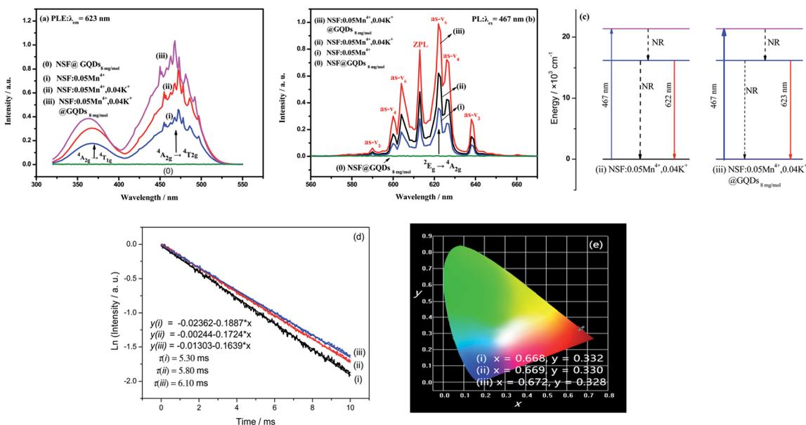
Fig. 3 Luminescent properties of four samples, (0) NSF@GQDs<sub>8 mg mol<sup>-1</sup></sub>, (i) NSF:0.05Mn<sup>4+</sup>, (ii) NSF:0.05Mn<sup>4+</sup>,0.04K<sup>+</sup>, and (iii) NSF:0.05Mn<sup>4+</sup>,0.04K<sup>+</sup>@GQDs<sub>8 mg mol<sup>-1</sup></sub>: (a) PLE spectra, (b) PL spectra, (c) diagram of energy level transition induced by GQDs, (d) decay curves, and (e) CIE chromaticity diagrams.
