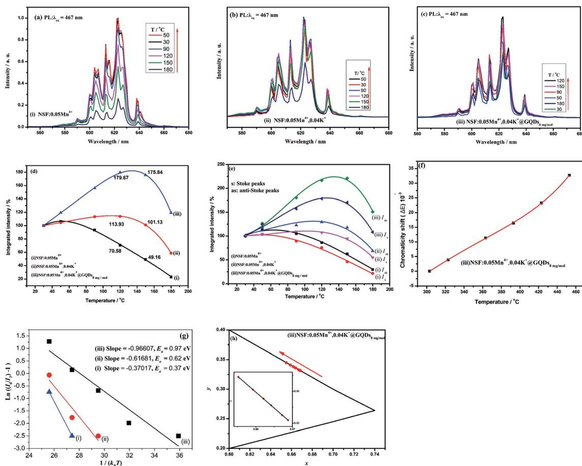
Fig. 5 PL performances of the three samples at different temperatures, (i) NSF:0.05Mn<sup>4+</sup>, (ii) NSF:0.05Mn<sup>4+</sup>,0.04K<sup>+</sup>, (iii) NSF:0.05Mn<sup>4+</sup>,0.04K<sup>+</sup>@GQDs<sub>8 mg mol<sup>-1</sup></sub>: (a), (b), and (c) PL spectra. (d) Integrated intensity curve. (e) Integrated intensity curves of Stoke and anti-Stoke peaks. (f) Chromaticity shift of sample (iii). (g)  $E_a$  curves. (h) CIE color coordinates of sample (iii).
