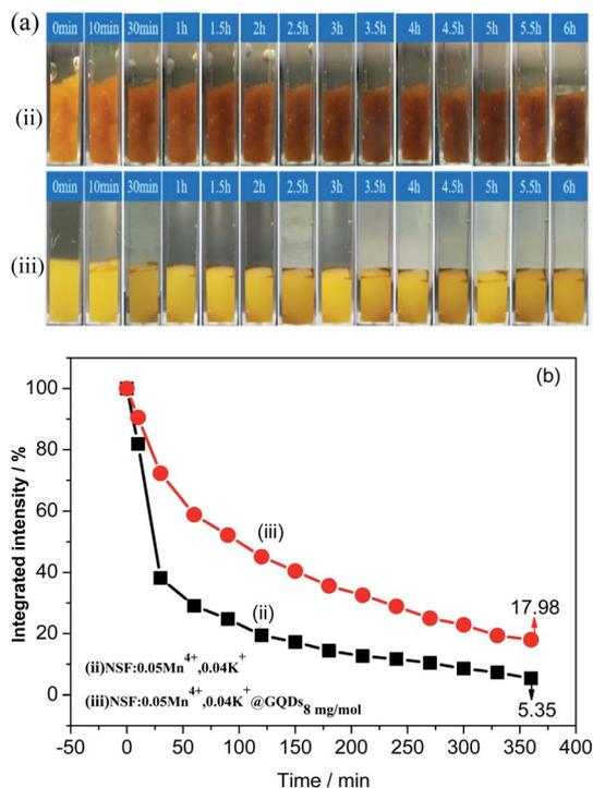
Fig. 7 Water resistance test of two samples: (ii) NSF:0.05Mn<sup>4+</sup>,0.04K<sup>+</sup> and (iii) NSF:0.05Mn<sup>4+</sup>,0.04K<sup>+</sup>@GQDs<sub>8 mg mol<sup>-1</sup></sub>: (a) photographs under natural light and (b) PL integrated intensities with different soaking times in water.
