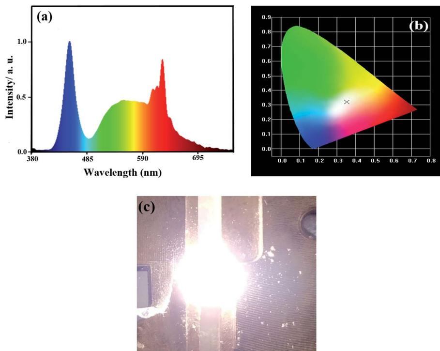
Fig. 8 Properties of prototype WLEDs fabricated using the mixed phosphors of NSF:0.05Mn<sup>4+</sup>,0.04K<sup>+</sup>@GQDs<sub>8</sub> mg mol<sup>-1</sup> and YAG:Ce<sup>3+</sup> based on an InGaN chip under a 20 mA drive current: (a) electroluminescence spectrum, (b) CIE chromaticity diagram and (c) luminescent photo.
