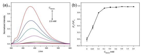
Fig. 3 (a) Fluorescence spectra of C-dots (0.035 mg mL $^{-1}$ ) in the presence of different concentrations of KMnO<sub>4</sub> (0, 0.05, 0.1, 0.2, 0.4, 0.6, 0.8, 1.0, 2.0 mM). (b) The plot of fluorescence quenching efficiency against the concentration of MnO<sub>2</sub> nanosheets.
