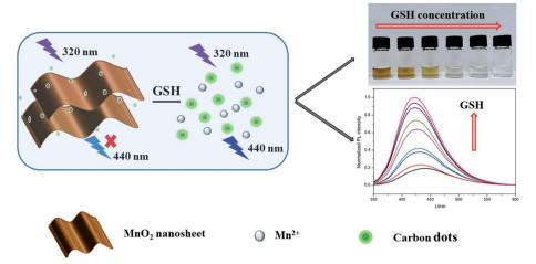
Scheme 1 Schematic illustration of the colorimetric and fluorescence dual-readout assay for GSH based on carbon dots $-MnO_2$  nanosheets platform.
