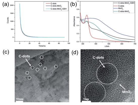
Fig. 2 (a) Fluorescence lifetime of C-dots, C-dots- $MnO_2$  nanosheets mixture, and C-dots- $MnO_2$  nanosheets mixture reacted with GSH. (b) The UV-Vis absorption spectra of C-dots,  $MnO_2$  nanosheets, C-dots- $MnO_2$  nanosheets mixture, and C-dots- $MnO_2$  nanosheets mixture reacted with GSH. (c) TEM image of C-dots- $MnO_2$  nanosheets mixture. (d) HRTEM image of C-dots- $MnO_2$  nanosheets mixture.
