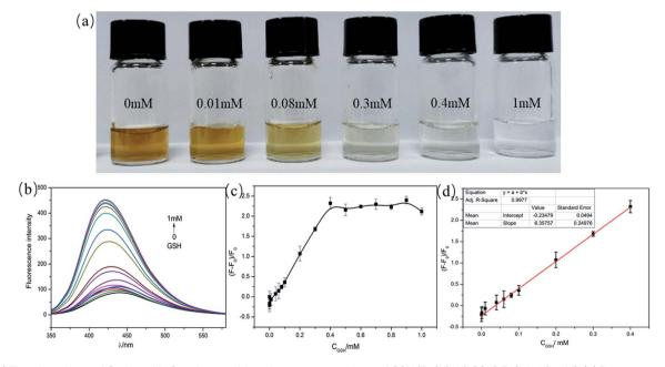
Fig. 4 (a) The photoshop of C-dots- $MnO_2$  mixture with various concentrations of GSH (0, 0.01, 0.08, 0.3, 0.4, 1.0 mM). (b) Fluorescence spectra of the C-dots- $MnO_2$  mixture in the presence of different concentrations of GSH (0, 0.1, 1, 10, 40, 60, 80  $\mu$ m and 0.1, 0.2, 0.3, 0.4, 0.5, 0.6, 0.7, 0.8, 0.9, 1.0 mM). (c) The relationship between the fluorescence recovery and the concentration of GSH. (d) The linear plot of fluorescence recovery *versus* the concentration of GSH.
