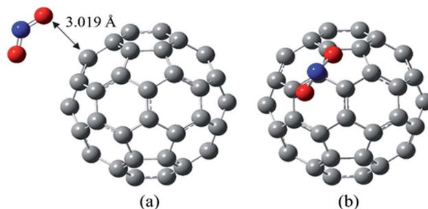
Fig. 1 The most stable complex of NO<sub>2</sub>/C<sub>60</sub> in two different views, at B97D/6-311G(d,p).
