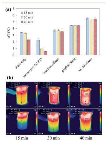
Fig. 4 (a) Temperature difference between the water surface and bottom and (b) IR images under irradiation: submerged AC-P25 (top) and AC-P25/foam (bottom).
