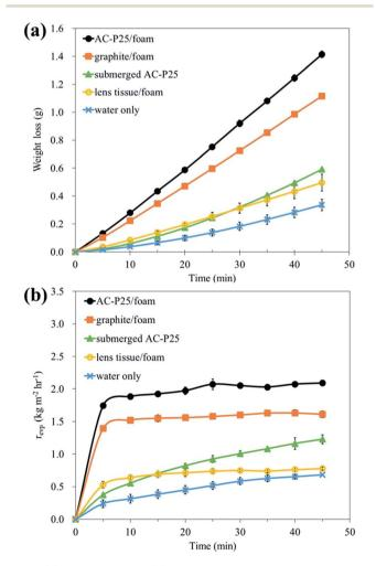
Fig. 3  $\,$  (a) Weight loss and (b) evaporation rates of different systems under irradiation.
