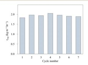
Evaporation rates for seven cycles using AC-P25/foam.
