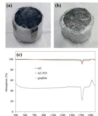
Fig. 1 Pictures of (a) AC-P25/foam and (b) graphite/foam. (c) UV-vis-NIR absorption spectra of the different photothermal layers.
