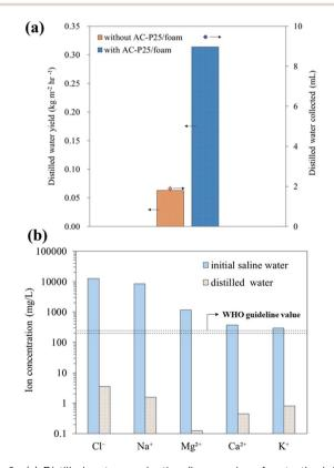
(a) Distilled water production (bar graph: refers to the left yaxis; diamond symbol: refers to the right y-axis) and (b) desalination ability using the solar still system with AC-P25/foam under outdoor sunlight irradiation
