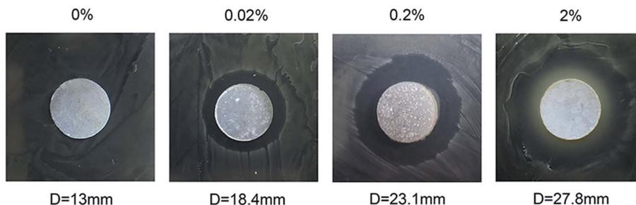
Fig. 7 Antibacterial activity of disc-like samples by the zone of inhibition (ZOI) test against *E. faecalis*.
