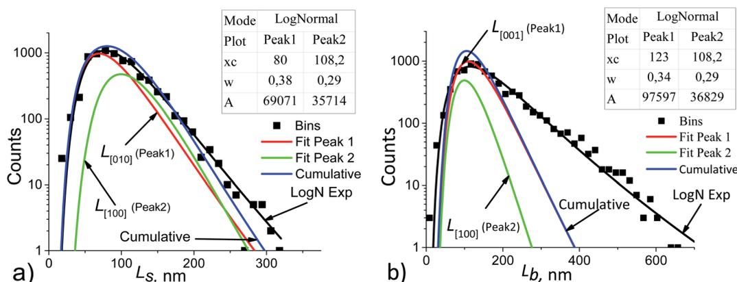
Fig. 5  $L_s$  (a) and  $L_b$  (b) particle size distribution histograms in sample no. 1 (black points) decomposed into the components. The basic parameters of the resulting LogNormal functions are shown in the insets using the notation of eqn (5).
