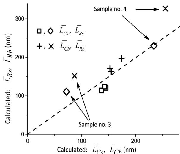
Fig. 4 Comparison  $\bar{L}_{R_s}$ ,  $\bar{L}_{R_b}$  and  $\bar{L}_{C_b}$ ,  $\bar{L}_{C_s}$  calculated by Approaches #2 and #3, respectively. The dashed line corresponds to their equality. The sizes of the points correspond approximately to the errors in the calculations (<10%) which result from the experimental errors.
