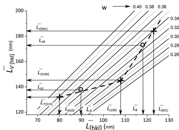
Fig. 6 Lognormal mean sizes  $L_{[hkl]}$  obtained by decomposing the TEM histograms into components and the volume-averaged sizes  $L_{V[hkl]}$  obtained directly from the XRD measurements. The family of straight lines is plotted for different  $w$  values (standard deviation of the lognormal function) in eqn (9).
