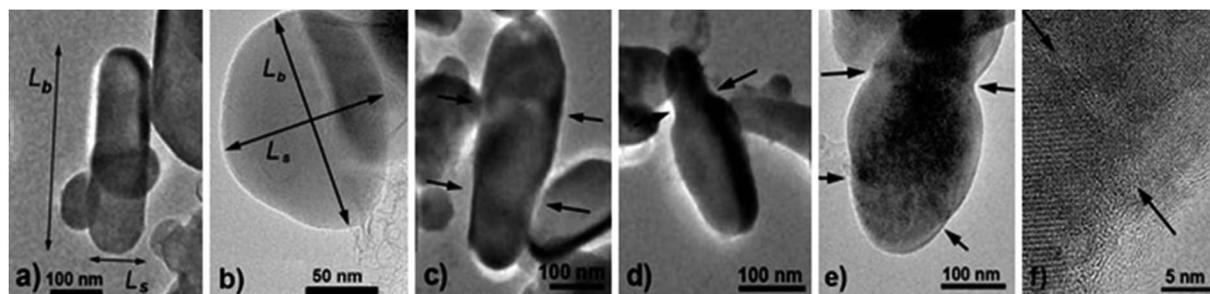
**Fig. 1** TEM images of LiFePO<sub>4</sub> powders in the samples: (a) no. 1, (b) no. 2. The measured width  $L_s$  and length  $L_b$  of the particle are shown with arrows. (c)–(e), (f) – fused and mosaic particles, respectively. The arrows show the boundaries between the blocks.
