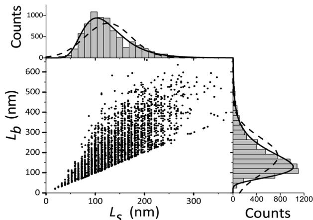
Fig. 2 Width  $L_s$  and length  $L_b$  of LiFePO<sub>4</sub> particles in sample no. 1. The corresponding frequency histograms are fitted with lognormal and Gaussian functions (solid and dashed lines, respectively).
