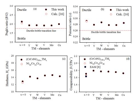
Fig. 5 The calculated (a) Pugh's ratio (b) Poisson's ratio (c) hardness and (d) compressibility of  $(CrCoNi)_{100-x}TM_x$  alloys.
