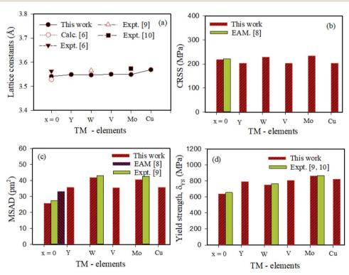
Fig. 2 The calculated (a) lattice constants (b) CRSS (c) MSAD and (d) yield strength of (NiCoCr)<sub>100-x</sub>TM<sub>x</sub> (TM = W, Mo, Y, V, Cu and x = 0, 4) MEAs.
