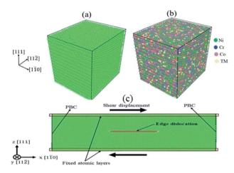
Fig. 1 Schematic diagram of (a)  $(CrCoNi)_{100-x}TM_x$  MEA with atoms colored according to the common neighbor analysis (CNA) method<sup>18</sup> in Open Visualization Tool  $(OVITO)^{19}$  to identify the fcc crystal structure (b) model after random initialization of Ni, Co, Cr, and TM (c) supercell with one edge dislocation.
