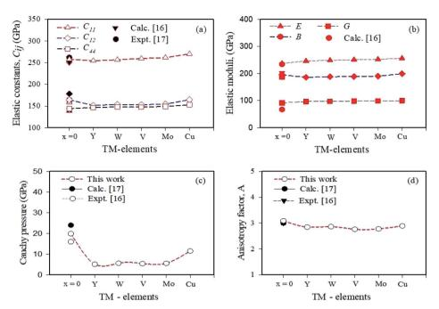
Fig. 4 The calculated (a) elastic constants (b) elastic moduli (c) Cauchy pressure and (d) anisotropy factor of (CrCoNi)<sub>100-x</sub>TM<sub>x</sub> alloys
