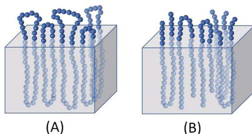
Fig. 8 Hypothetical illustration of the smoothed surface of crystallites consisting of cyclic polyLA (A) or of linear polyLA (B).
