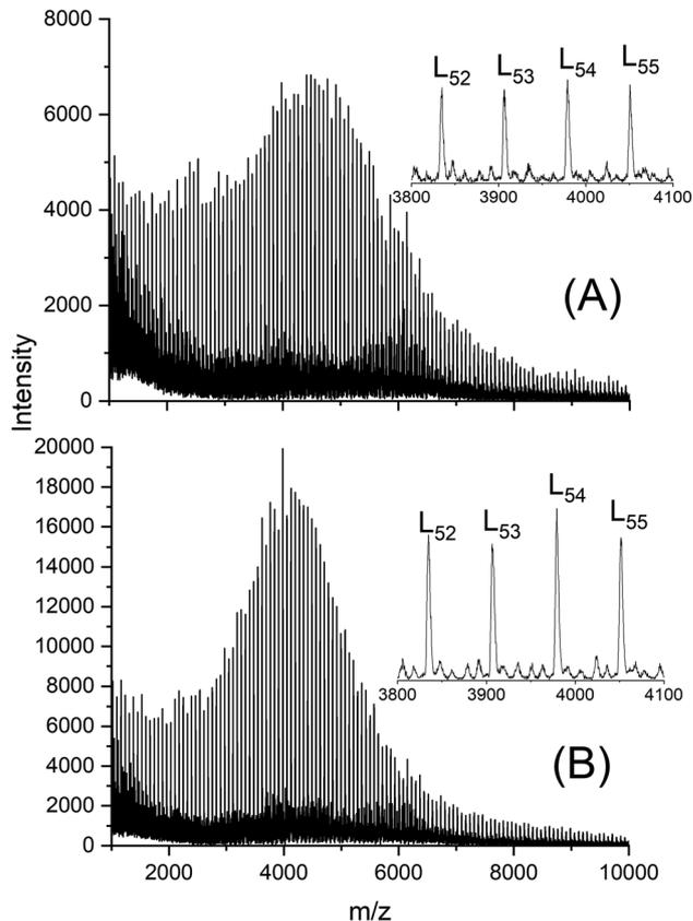
Fig. 4 MALDI TOF mass spectra of ethyl lactate-initiated polylactides polymerized with (A) SnBiph at 150 °C/1 d (No. 2, Table 5), (B) SnOct<sub>2</sub> at 140 °C/1 d (No. 7, Table 5). L = linear chains having ethyl ester end groups.
