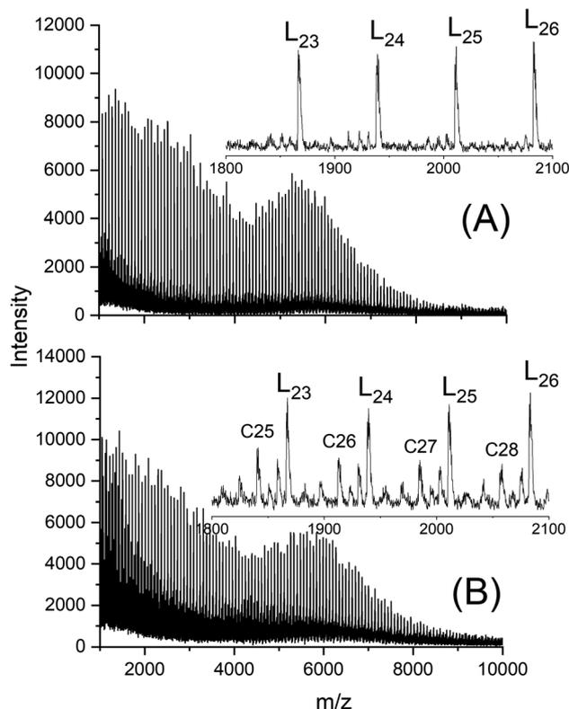
Fig. 5 MALDI TOF mass spectra of polylactides initiated with 11-undecenol and catalyzed with SnBiph at 160 °C: (A) LA/In = 100/1, No. 4 Table 2, (B) LA/In = 200/1, No. 5, Table 2. L = linear chains having undecenyl ester end groups.
