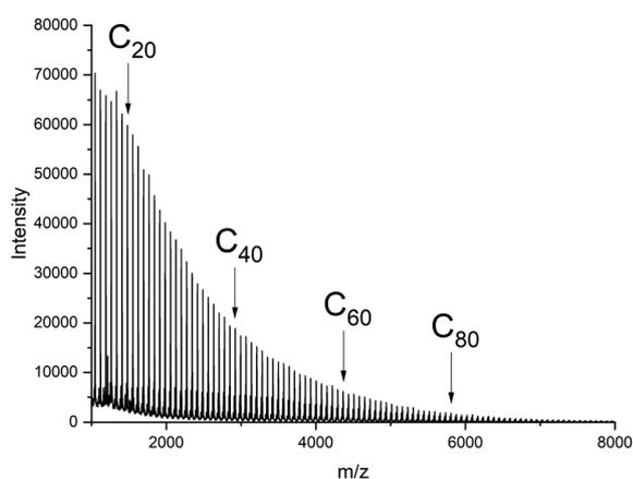
Fig. 6 MALDI TOF mass spectrum of a polylactides prepared with  $\text{Ph}_2\text{SnCl}_2$  as catalyst in bulk at 160 °C/1 h (reproduced from ref. 23).
