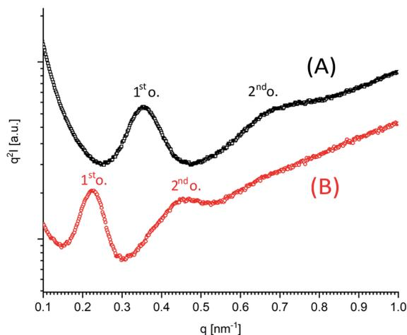
Fig. 7 SAXS Kratky plots of poly(lactides) prepared with ethyl lactate as initiator and with: (A) SnOct<sub>2</sub> as catalyst at 130 °C (No. 8, Table 5), (B) SnBiph as catalyst at 160 °C (No. 1, Table 5), 1<sup>st</sup> o. = reflection of first order of lamellar long period *L*.
