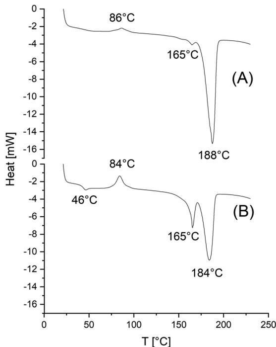
Fig. 3 DSC heating traces of polyLA prepared with SnOct<sub>2</sub> as catalyst and 1-HMN as initiator (LA/In = 100/1) at 160 °C, 3 d: (A) after 1 h (No. 9, Table 4), (B) after 0.5 h (No. 8, Table 4).
