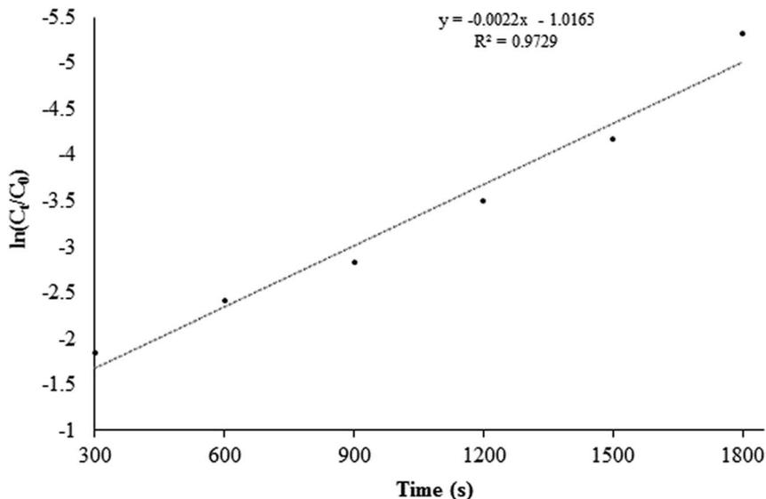
Fig. 6 A pseudo-first-order plot for photocatalytic Cr(vi) reduction catalyzed by STA-12-Mn-Fe (50 : 50).
