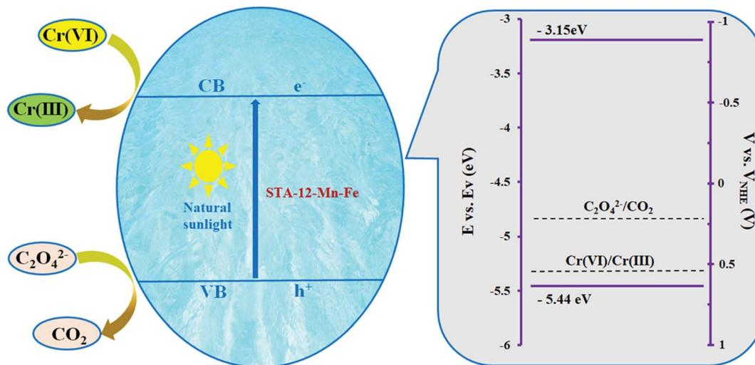
Fig. 8 A schematic diagram of Cr(vi) removal with the STA-12-Mn-Fe (50 : 50) photocatalyst under visible light irradiation.
