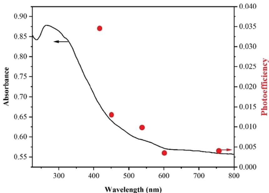
Fig. 5 The absorption spectrum of STA-12-Mn-Fe (50 : 50) (solid line) and action spectrum for the removal of Cr(vi) in the optimal situation under CFL radiation (red points).
