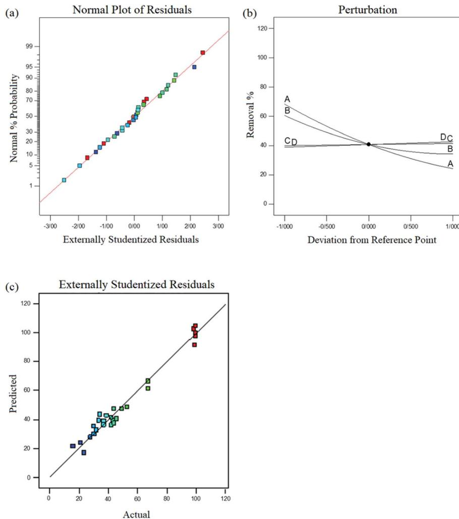
Fig. 2 (a) Residuals in the normal probability plot. (b) A perturbation plot for the removal of Cr(vi) over STA-12-Mn-Fe (50 : 50). (c) Actual data vs. predicted data for Cr(vi) reduction.
